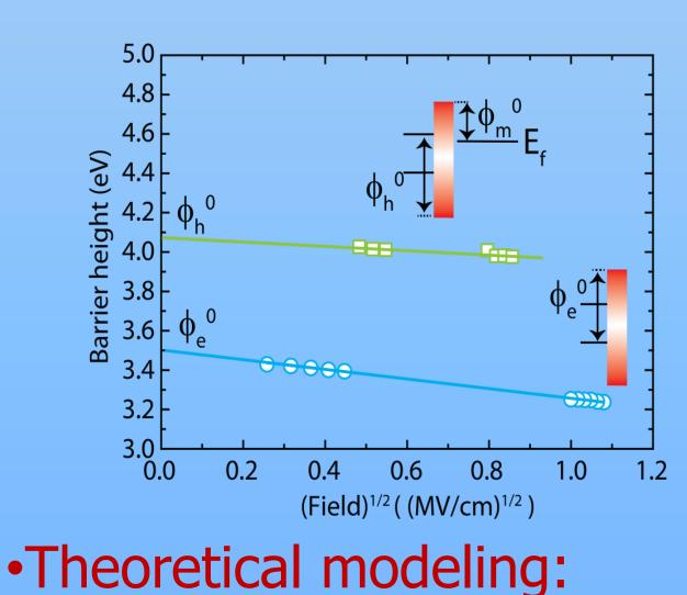
Considering the Schottky barrier lowering effect, the zero barrier height can be achieved by extrapolating the barrier heights under various electric fields. The electron and hole barrier heights are shown to be 3.5 eV and 4.1 eV. Then E<sub>g</sub>(Al<sub>2</sub>O<sub>3</sub>) is 6.5 eV.
