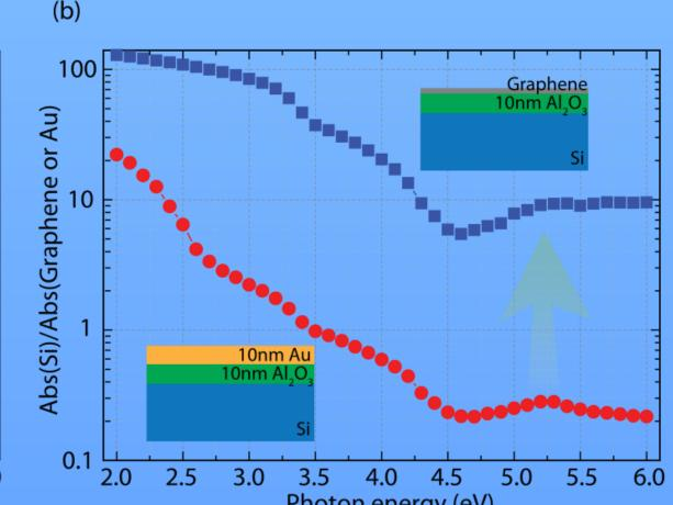
Using thin film optics, we calculate the absorption by graphene and show the advantage of using graphene as transparent contact.
