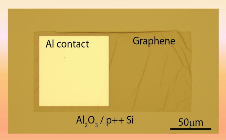
➤ Large-area CVD-growth graphene is transferred to the 10 nm ALD Al<sub>2</sub>O<sub>3</sub> covered p++ Si substrate, followed by oxygen plasma etching to pattern a 100 x 200 µm<sup>2</sup> rectangular
