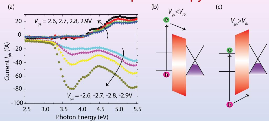
➤ Photocurrents are recorded as a function of incident photon energy. The positive and negative currents are respectively related to hole and electron injections from Si into oxide.
