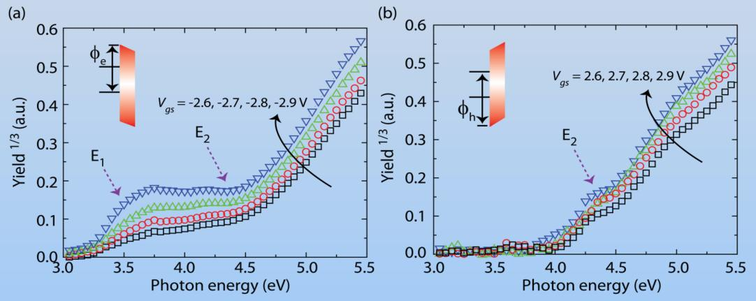
To extract the barrier heights, quantum yield (Y) is determined using the currents normalized by the incident light power.
