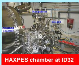
Non-destructive analysis of chemical & electronic properties of buried layers and interfaces
