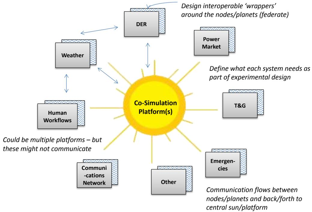
**Figure 5-7. Layers for Co-Simulation Platform Approach**
