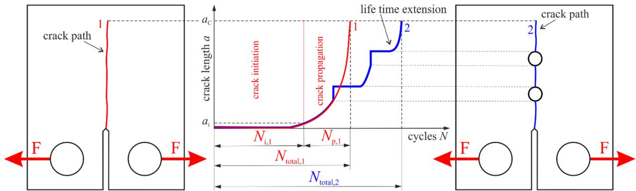
Figure 1 Manipulation of life time caused by notches - schematic illustration
