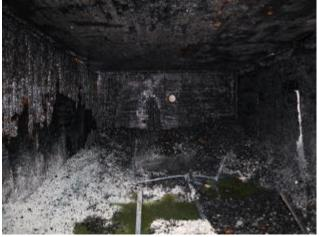
(a) interior of CLT compartment after Test 1-5
