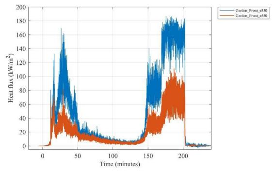
Figure I 15. Heat flux measured by Gardon gauges 350 cm and 550 cm above the floor above the doorway.
