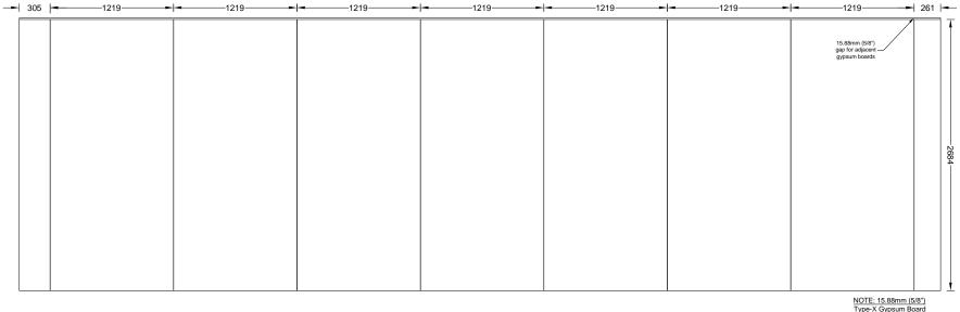
Type-X Gypsum Board Fastened w/ 41mm (1 5/8") Type-S Drywall Screws Used
