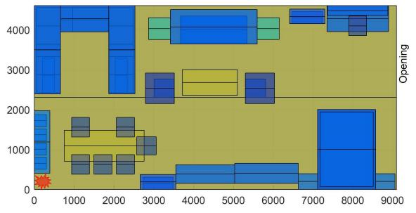
Figure 11. Plan view of a model of the moveable fuel as installed (units in mm).
