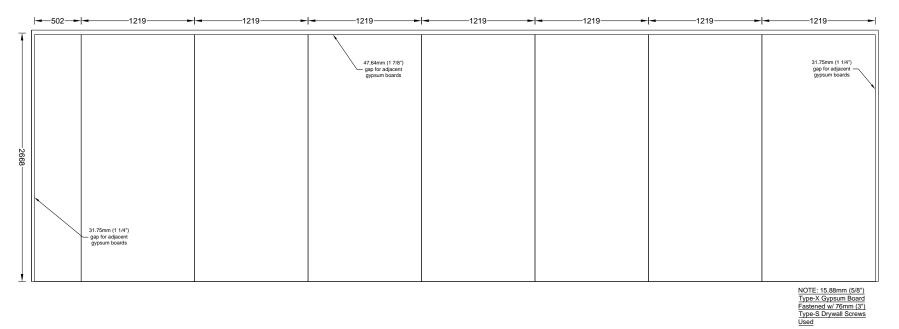
Figure A 37. Test 1-2 Large Compartment CLT - W1 - Gypsum Layout - Face Layer
