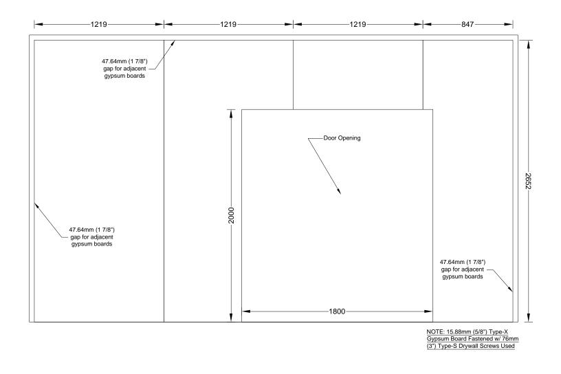
Figure A 74. Test 1-4 Large Compartment CLT - W2 - Gypsum Layout - Face Layer
