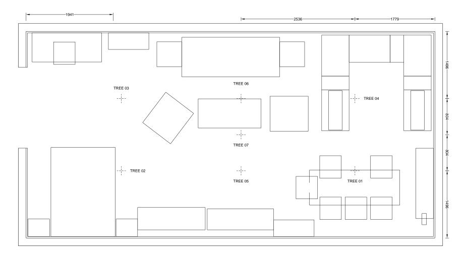
Figure A 87. Test 1-5 Large Compartment CLT - Instrumentation Tree Layout
