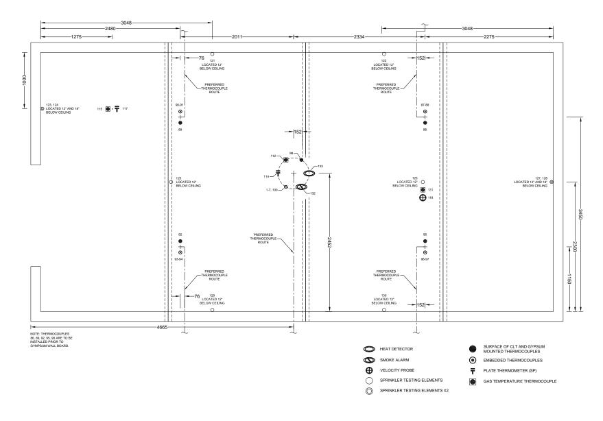
Figure A 102. Test 1-6 Large Compartment CLT - Ceiling - Instrumentation Layout
