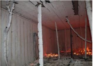
(e) at 130 min – near end of test, gypsum board remained: 2 layers on ceiling; 3 layers on walls
