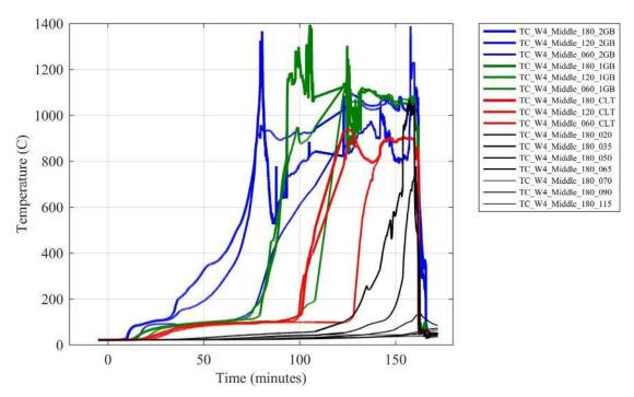
Figure J 13. Temperatures in Wall W4 at various depths from the fire exposed surface.
