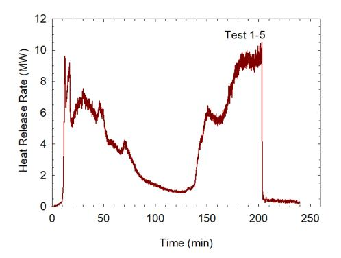
Figure 83. Heat release rate during Test 1-5 (test terminated at 202 min).
