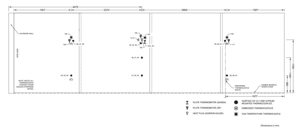
Figure 23. Measurement devices in W1 wall.
