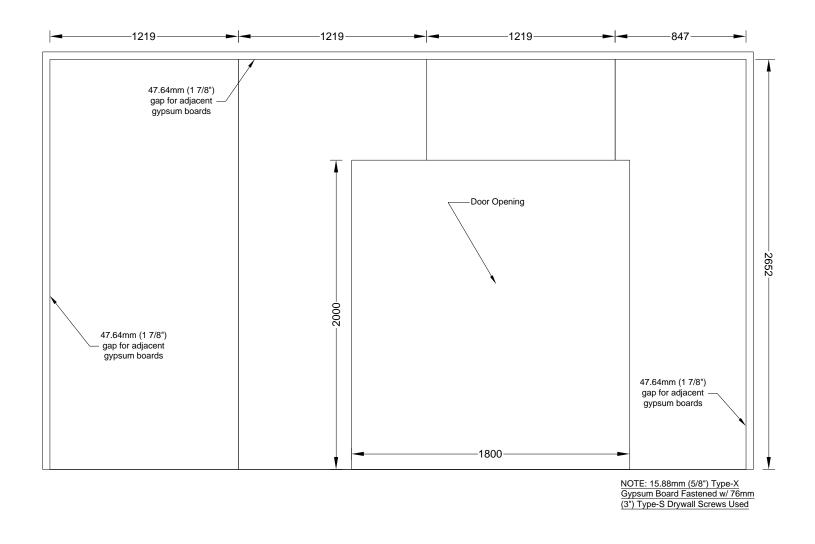
Figure A 95. Test 1-5 Large Compartment CLT - W2 - Gypsum Layout - Face Layer
