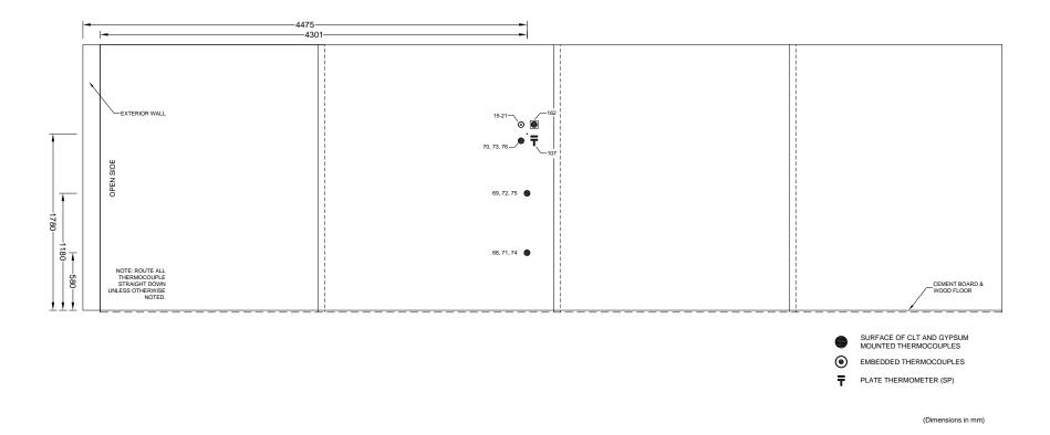
Figure A 84. Test 1-5 Large Compartment CLT - W3 - Instrumentation Layout
