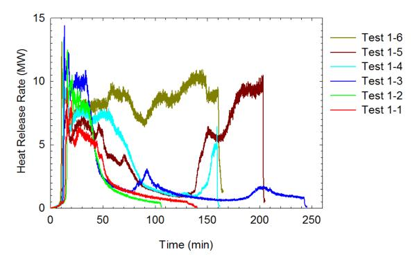
Figure 103. Heat release rates in CLT compartment tests.
