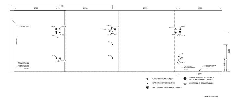
Figure A 103. Test 1-6 Large Compartment CLT - W1 - Instrumentation Layout
