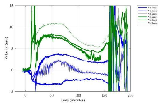
Figure H 28. Gas velocities measured in the doorway (positive indicates flow out the door). [10 s moving average filter applied]
