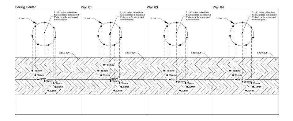
Figure A 86. Test 1-5 Large Compartment CLT - Embedded Thermocouple Detail
