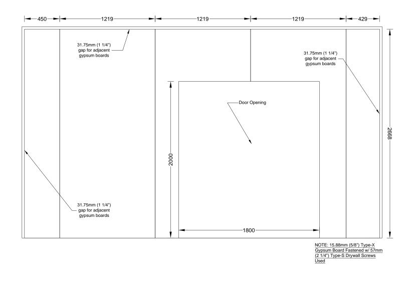
Figure A 111. Test 1-6 Large Compartment CLT - W2 - Gypsum Layout - Middle Layer
