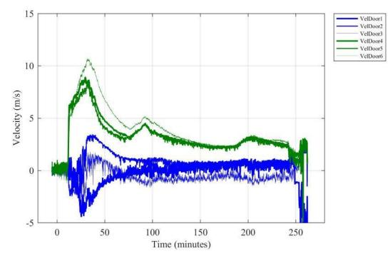
Figure G 28. Gas velocities measured in the doorway (positive indicates flow out the door). [10 s moving average filter applied]
