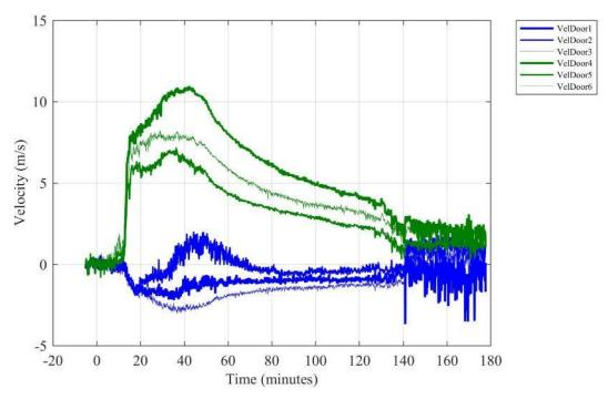
Figure E 31. Gas velocities measured in the doorway (positive indicates flow out the door). [10 s moving average filter applied]
