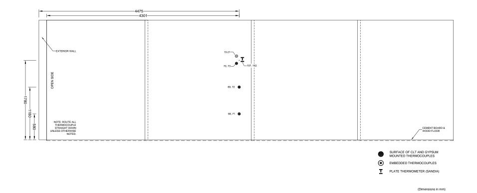
Figure A 28. Test 1-2 Large Compartment CLT - W3 - Instrumentation Layout
