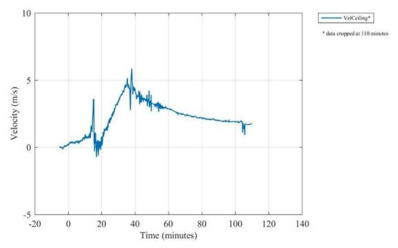
Figure F 30. Gas velocity measured 305 mm from the ceiling along the midline 227.5 cm from the back of the compartment (positive indicates flow out the door). [10 s moving average filter applied]
