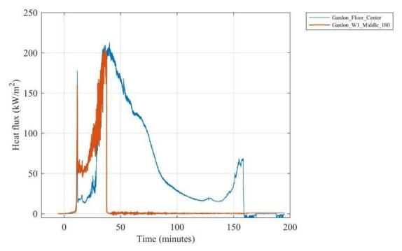
Figure H 14. Heat flux measured by Gardon gauges located inside the compartment.
