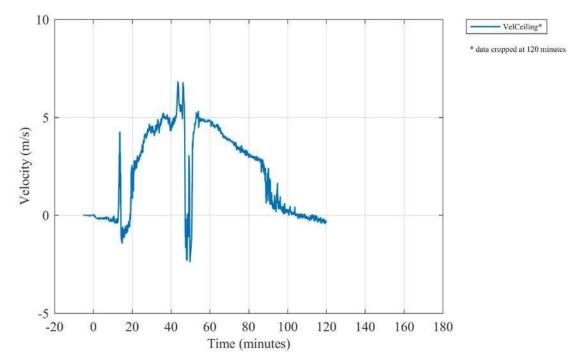
Figure E 30. Gas velocity measured 305 mm from the ceiling along the midline 227.5 cm from the back of the compartment (positive indicates flow out the door). [10 s moving average filter applied]
