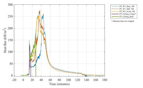
Figure E 17. Heat flux calculated from plate thermometers at various locations inside the compartment.
