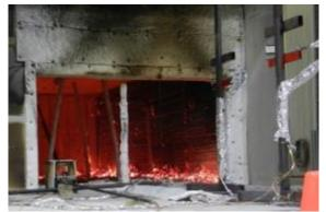
(e) exposed W1 at 120 min after 1<sup>st</sup> ply falling off
