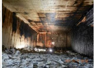
(b) W3, W4 W1 and ceiling CLT after Test 1-3.
