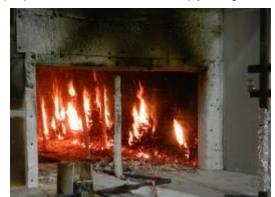
(f) exposed W1 at 190 min before 2<sup>nd</sup> ply falling off
