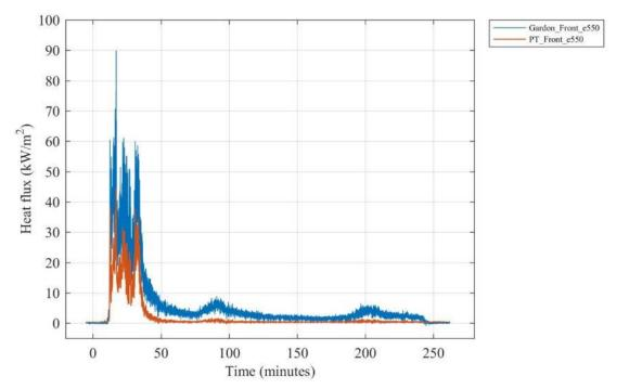
Figure G 21. Comparison of heat fluxes recorded by a collocated Gardon gauge and plate thermometer (PT) 350 cm above the floor above the doorway.
