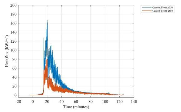
Figure F 15. Heat flux measured by Gardon gauges 350 cm and 550 cm above the floor above the doorway.
