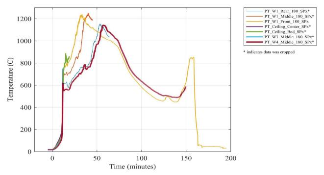
Figure H 29. Plate thermometer temperatures at various locations inside the compartment.
