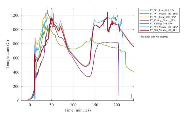
Figure I 29. Plate thermometer temperatures at various locations inside the compartment.
