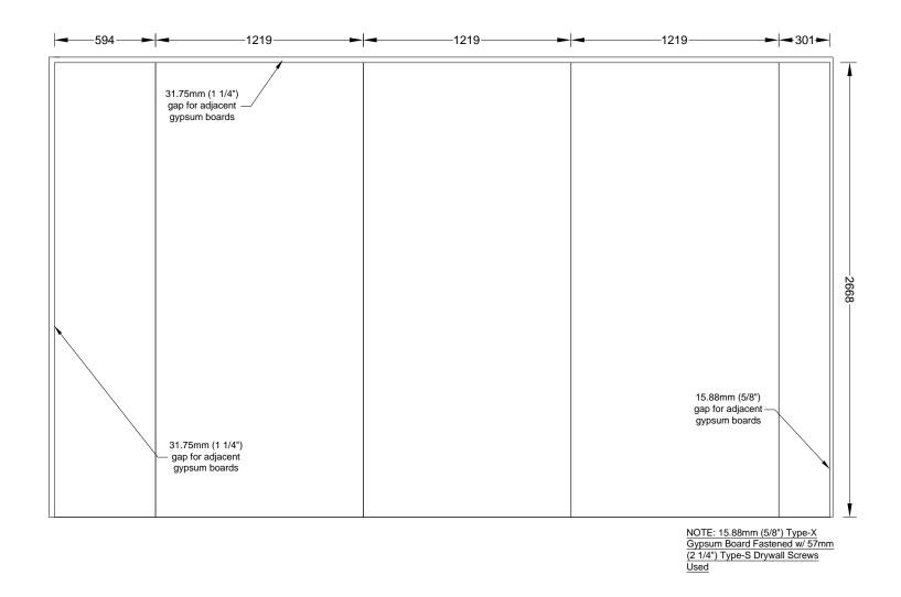
Figure A 22. Test 1-1 Large Compartment CLT - W4 - Gypsum Layout - Middle Layer
