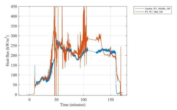
Figure J 20. Comparison of heat fluxes recorded by a collocated Gardon gauge, plate thermometer (PT) and differential flame thermometer (DFT) on Wall W1 at the middle of the compartment 1.8 m above the floor.
