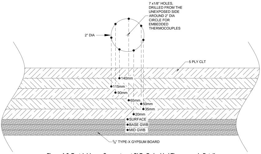
Figure A 5. Test 1-1 Large Compartment CLT - Embedded Thermocouple Detail
