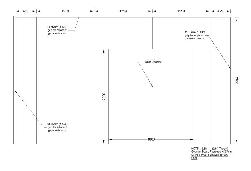
Figure A 94. Test 1-5 Large Compartment CLT - W2 - Gypsum Layout - Middle Layer
