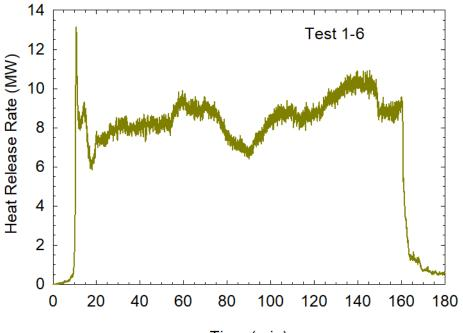
Time (min) Figure 97. Heat release rate during Test 1-6 (test terminated at 160 min).
