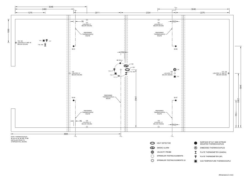
Figure A 1. Test 1-1 Large Compartment CLT - Ceiling - Instrumentation Layout
