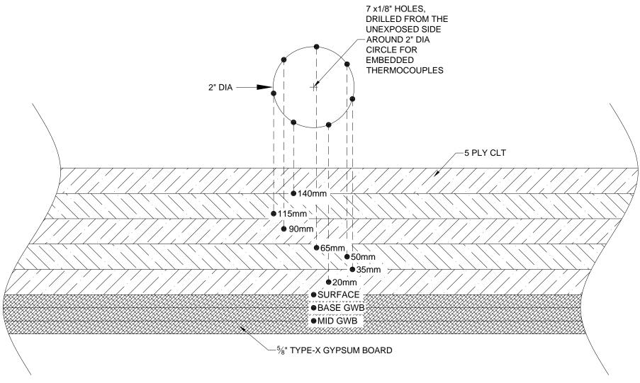
Figure 26. Details of embedded thermocouples in ceiling and walls with the drilled holes sealed from the outside (additional thermocouples added at the 2<sup>nd</sup> and 3<sup>rd</sup> gluelines in Test 1-5 and Test 1-6).
