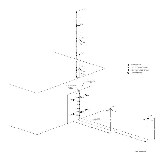
Figure A 109. Test 1-6 Large Compartment CLT - Exterior Instrumentation Layout
