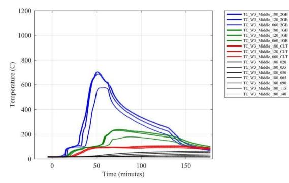
Figure E 12. Temperatures in Wall W3 at various depths from the fire exposed surface.
