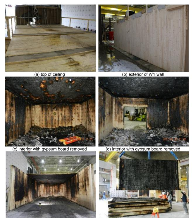
(e) during demolition (f) ceiling panels Figure 77. Photograph of CLT compartment and panels after Test 1-4.
