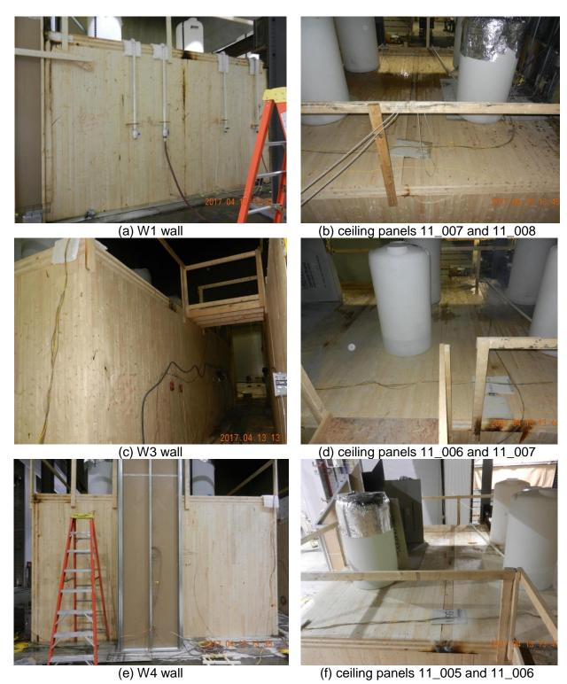
Figure 87. Exterior surface and joints of CLT compartment after Test 1-5.
