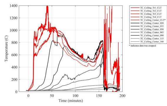
Figure H 10. Temperatures in the ceiling at various depths from the fire exposed surface.
