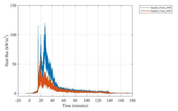
Figure E 15. Heat flux measured by Gardon gauges 350 cm and 550 cm above the floor above the doorway.
