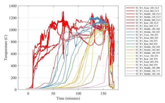
Figure J 11. Temperatures in Wall W1 at various depths from the fire exposed surface.
