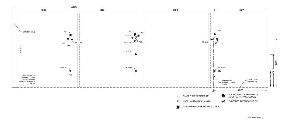
Figure A 62. Test 1-4 Large Compartment CLT - W1 - Instrumentation Layout
