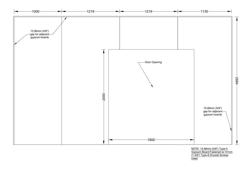
Figure A 110. Test 1-6 Large Compartment CLT - W2 - Gypsum Layout - Base Layer
