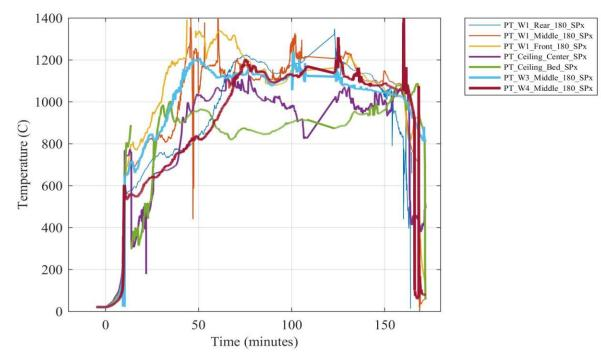
Figure J 29. Plate thermometer temperatures at various locations inside the compartment.
