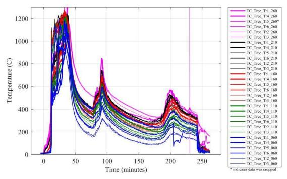
Figure G 8. Thermocouple tree temperatures at various locations inside the compartment.
