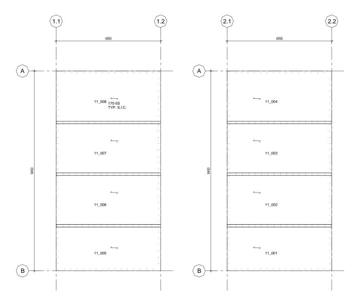
Figure 3. Ceiling Panels of CLT Compartments.
