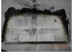
(c) middle block near TC Tree 6 charred 45 mm (d) rear block near TC Tree 4 charred 42 mm Figure 46. Char of small CLT blocks in Test 1-1 (cut to half to show remaining thickness).
