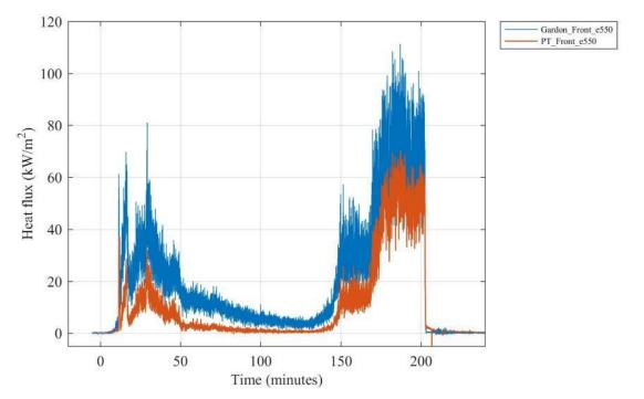
Figure I 22. Comparison of heat fluxes recorded by a collocated Gardon gauge and plate thermometer (PT) 550 cm above the floor above the doorway.
