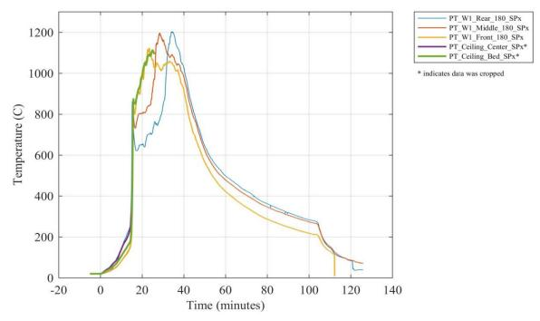
Figure F 32. Plate thermometer temperatures at various locations inside the compartment.
