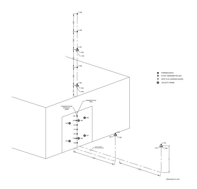
Figure A 89. Test 1-5 Large Compartment CLT - Exterior Instrumentation Layout
