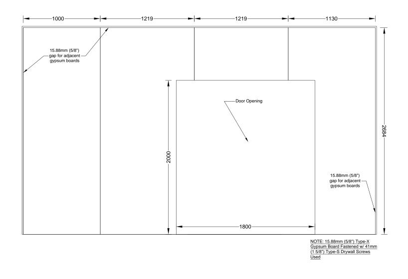
Figure A 93. Test 1-5 Large Compartment CLT - W2 - Gypsum Layout - Base Layer
