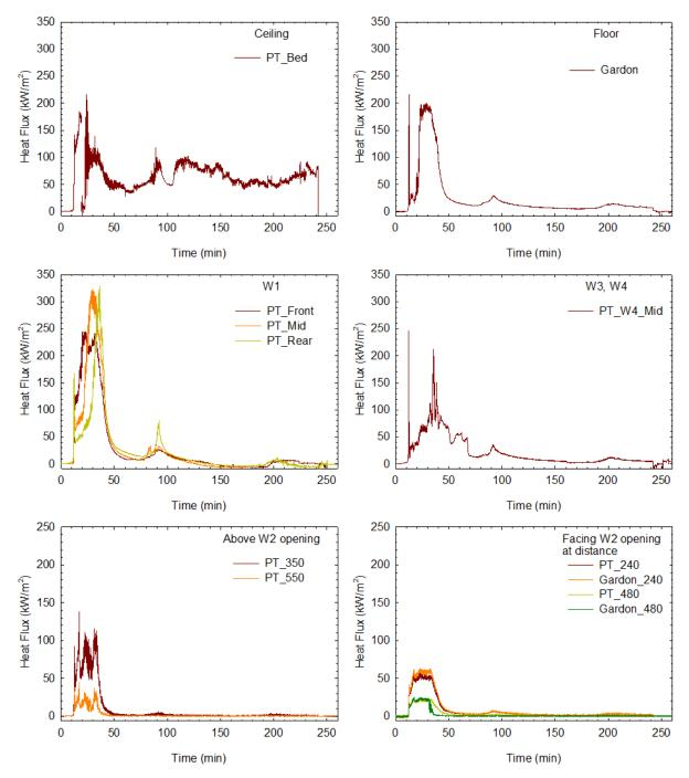
Figure 65. Heat fluxes inside and outside the compartment during Test 1-3 (test terminated at 242 min).
