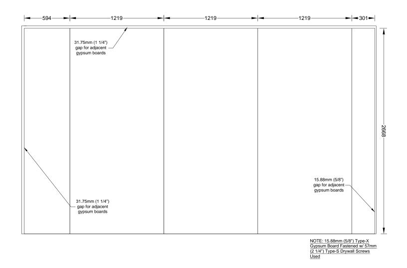
Figure A 79. Test 1-4 Large Compartment CLT - W4 - Gypsum Layout - Middle Layer
