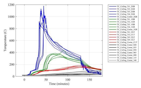
Figure E 10. Temperatures in the ceiling at various depths from the fire exposed surface.
