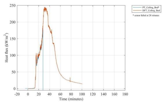
Figure E 23. Comparison of heat fluxes recorded by a collocated plate thermometer (PT) and differential flame thermometer (DFT) on the ceiling above the bed.
