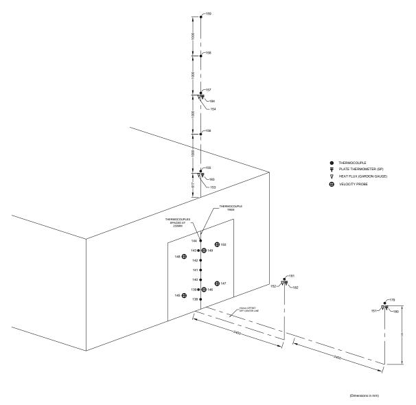
Figure A 8. Test 1-1 Large Compartment CLT - Exterior Instrumentation Layout
