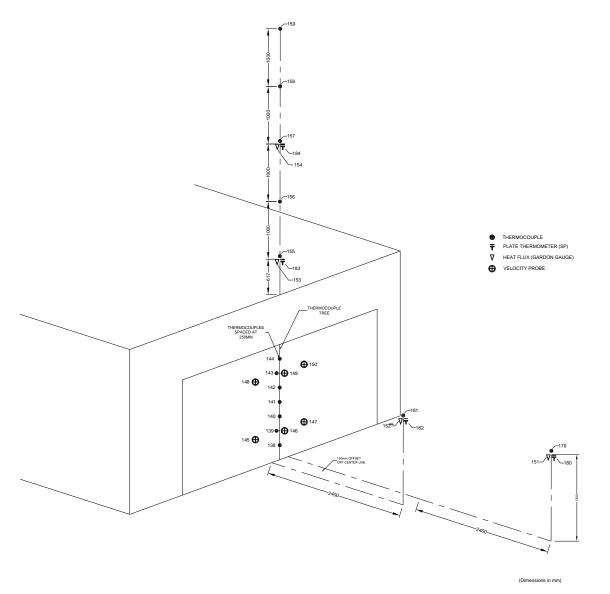
Figure A 51. Test 1-3 Large Compartment CLT - Exterior Instrumentation Layout
