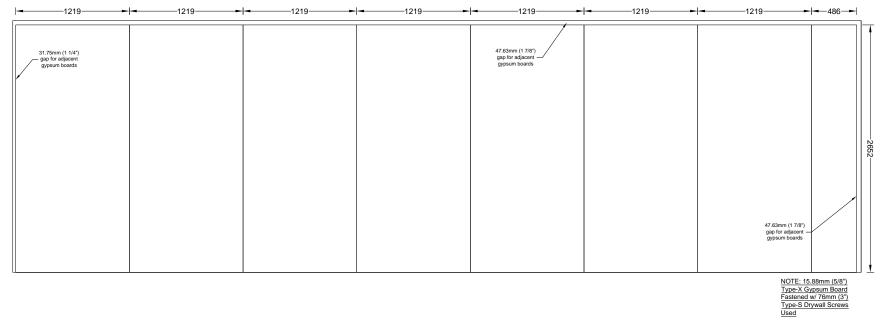
Figure A 115. Test 1-6 Large Compartment CLT - W3 - Gypsum Layout - Face Layer
