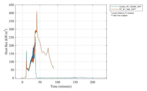
Figure I 20. Comparison of heat fluxes recorded by a collocated Gardon gauge, plate thermometer (PT) and differential flame thermometer (DFT) on Wall W1 at the middle of the compartment 1.8 m above the floor.
