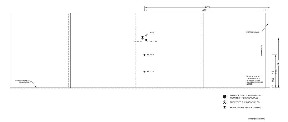
Figure A 3. Test 1-1 Large Compartment CLT - W3 - Instrumentation Layout
