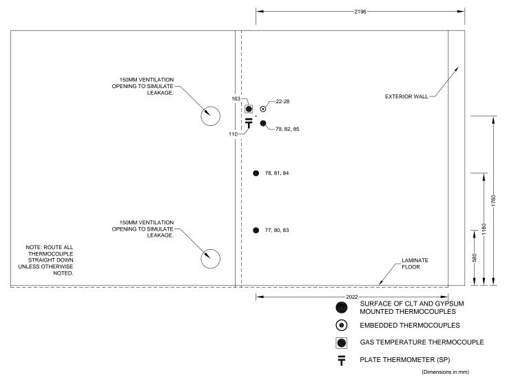
Figure A 64. Test 1-4 Large Compartment CLT - W4 - Instrumentation Layout
