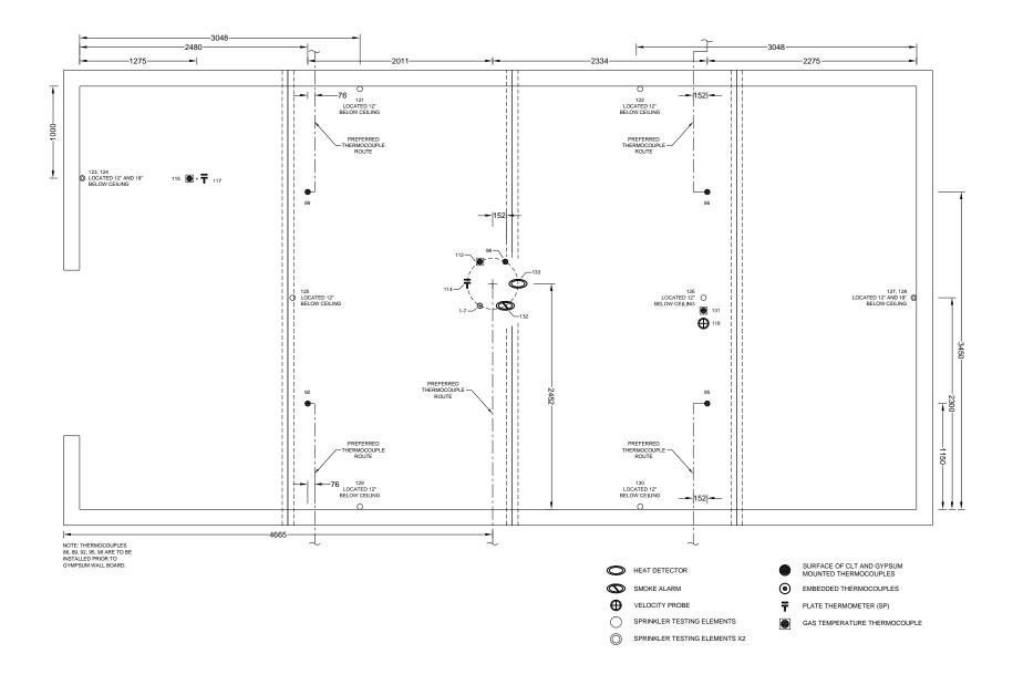
Figure A 61. Test 1-4 Large Compartment CLT - Ceiling - Instrumentation Layout
