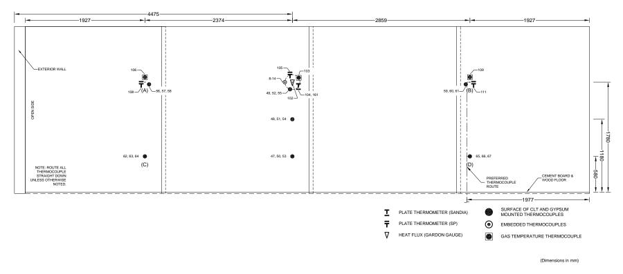
Figure A 2. Test 1-1 Large Compartment CLT - W1 - Instrumentation Layout
