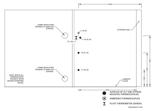
Figure 25. Measurement devices in W4 wall.
