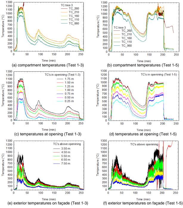
Figure 91. Effect of ventilation – Temperatures in Test 1-3 and Test 1-5.
