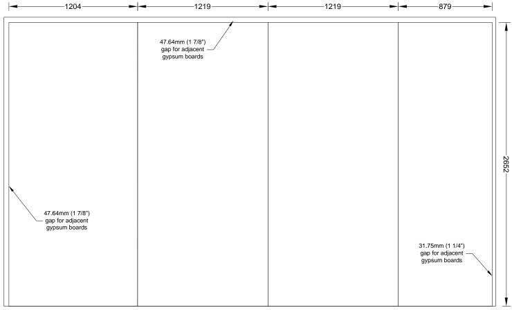
NOTE: 15.88mm (5/8") Type-X Gypsum Board Fastened w/ 76mm (3") Type-S Drywall Screws Used
