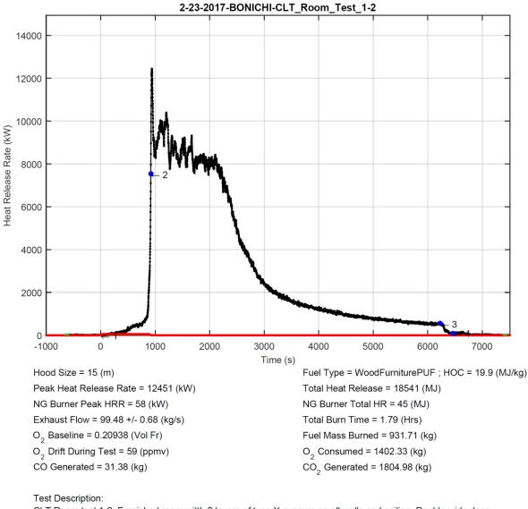
CLT Room test 1-2. Furnished room witth 2 layers of type X gypsum on all walls and ceiling. Double wide door opening
