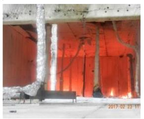
(e) at 100 min – near end of test, gypsum board remained: base layer on ceiling; 2 layers on walls
