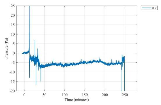
Figure G 26. Differential room pressure measured 210 cm above the floor at the center of the compartment.
