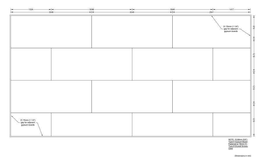
Figure A 92. Test 1-5 Large Compartment CLT - Ceiling - Gypsum Layout - Face Layer
