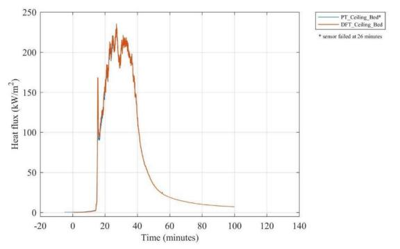
Figure F 23. Comparison of heat fluxes recorded by a collocated plate thermometer (PT) and differential flame thermometer (DFT) on the ceiling above the bed.
