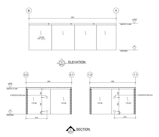
Figure 4. Elevation and Section View of CLT Compartments.
