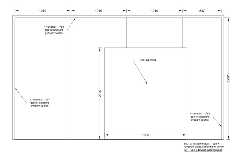
Figure A 112. Test 1-6 Large Compartment CLT - W2 - Gypsum Layout - Face Layer
