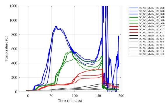
Figure H 12. Temperatures in Wall W3 at various depths from the fire exposed surface.
