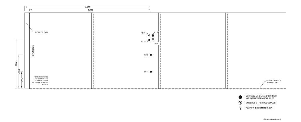
Figure A 46. Test 1-3 Large Compartment CLT - W3 - Instrumentation Layout
