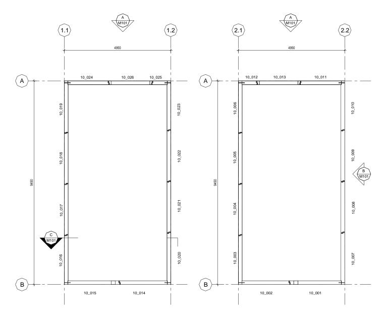
Figure 2. Wall Panels of CLT Compartments.
