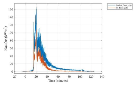
Figure F 24. Comparison of heat fluxes recorded by a collocated Gardon gauge and plate thermometer (PT) 350 cm above the floor above the doorway.
