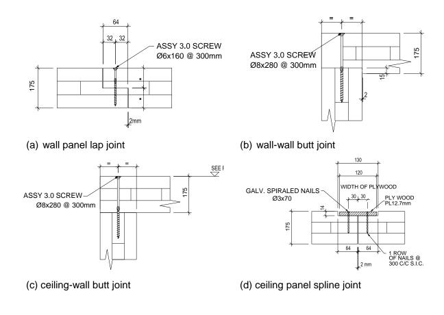
Figure 6. Details of CLT Panel Connections.
