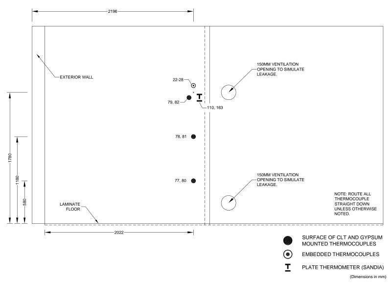
Figure A 29. Test 1-2 Large Compartment CLT - W4 - Instrumentation Layout
