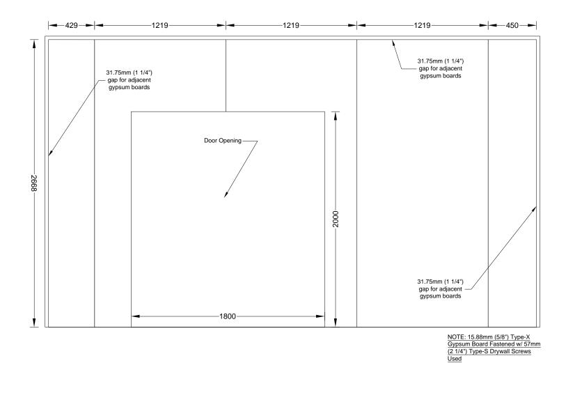
Figure A 16. Test 1-1 Large Compartment CLT - W2 - Gypsum Layout - Middle Layer
