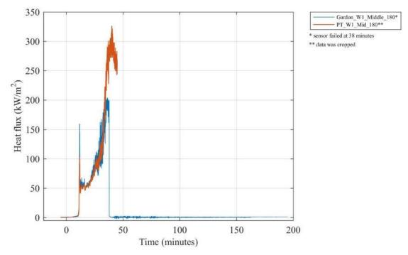
Figure H 20. Comparison of heat fluxes recorded by a collocated Gardon gauge, plate thermometer (PT) and differential flame thermometer (DFT) on Wall W1 at the middle of the compartment 1.8 m above the floor.
