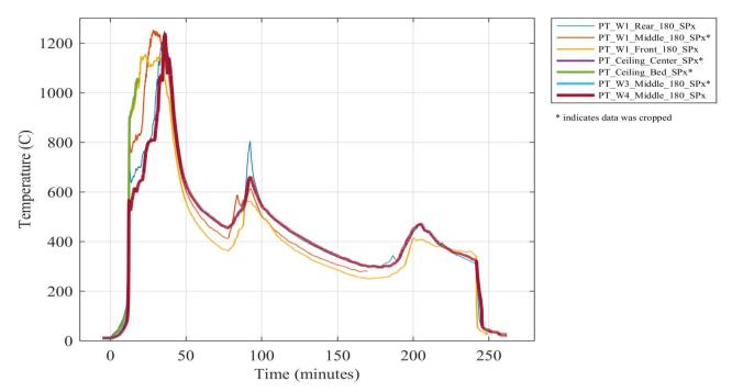
Figure G 29. Plate thermometer temperatures at various locations inside the compartment.
