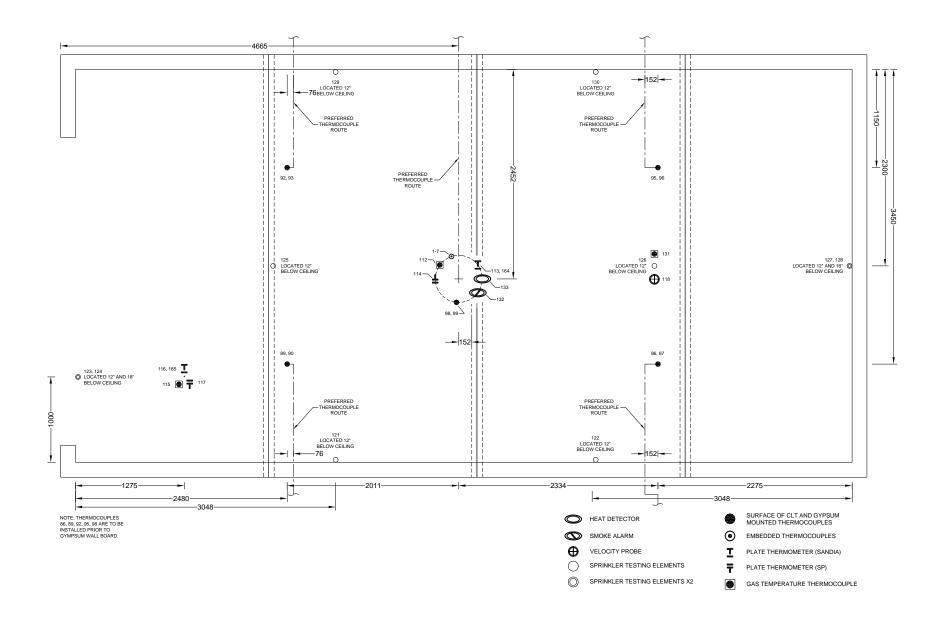
Figure A 26. Test 1-2 Large Compartment CLT - Ceiling - Instrumentation Layout
