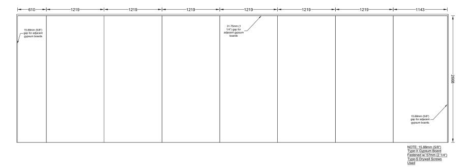
Figure A 70. Test 1-4 Large Compartment CLT - W1 - Gypsum Layout - Middle Layer
