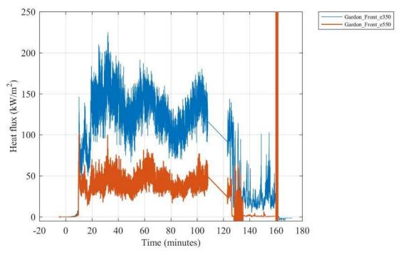
Figure J 15. Heat flux measured by Gardon gauges 350 cm and 550 cm above the floor above the doorway.
