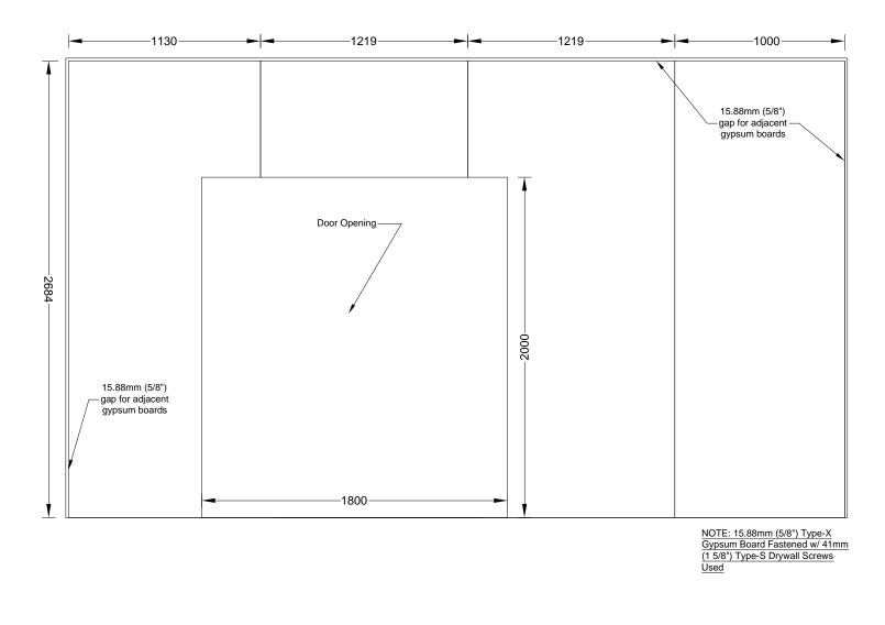
Figure A 15. Test 1-1 Large Compartment CLT - W2 - Gypsum Layout - Base Layer
