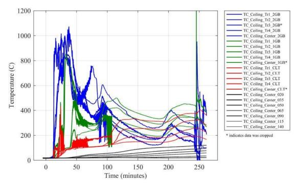
Figure G 10. Temperatures in the ceiling at various depths from the fire exposed surface.
