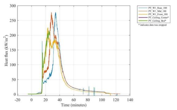
Figure F 17. Heat flux calculated from plate thermometers at various locations inside the compartment.
