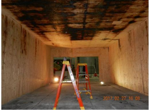
(b) CLT structure after repair Figure 60. Photographs of CLT structure before Test 1-3.
