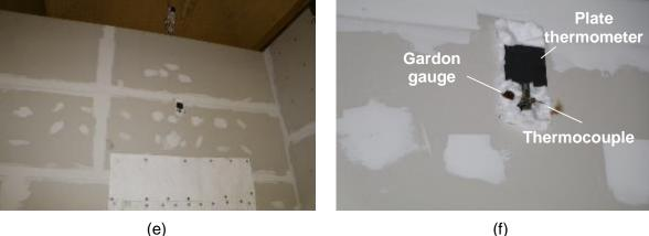
Figure 36. Photographs of heat flux sensors: (a) plate thermometer on wall inside compartment, (b) co-located Gardon gauge, plate thermometer and differential flame thermometer on wall inside compartment, (c) heat flux sensors on stands facing the doorway, (d) detail of heat flux sensors facing the doorway, (e) heat flux sensors in the wall above the doorway and (f) detail of heat flux sensors above the doorway.
