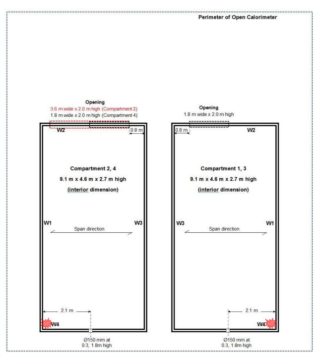
Figure 1. Schematic of test compartments.
