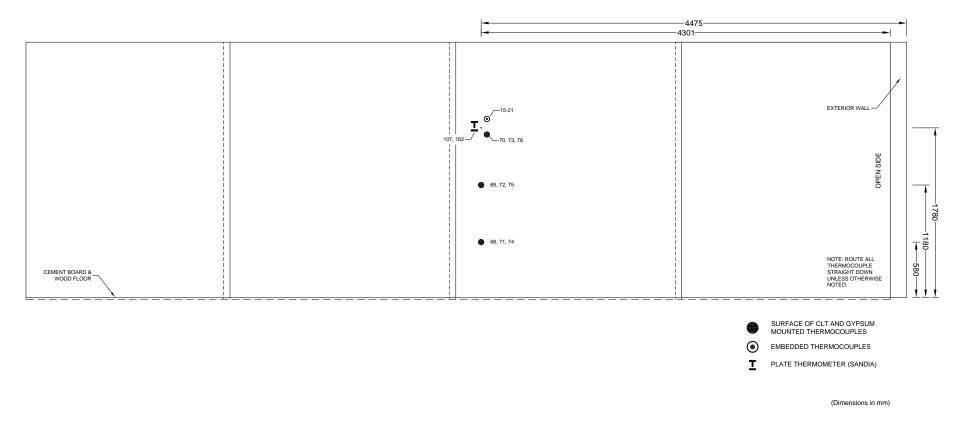
Figure 24. Measurement devices in W3 wall.
