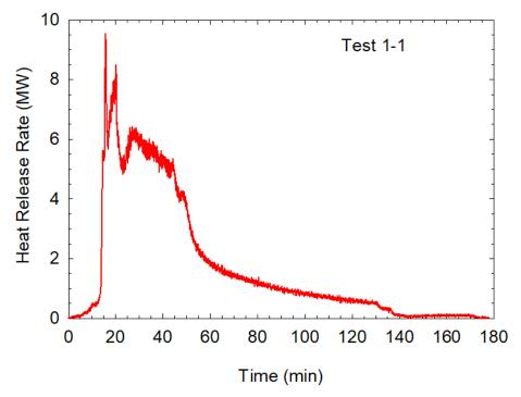
Figure 43. Heat release rate during Test 1-1 (test terminated at 134 min).
