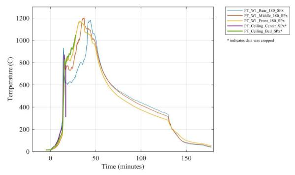
Figure E 32. Plate thermometer temperatures at various locations inside the compartment.
