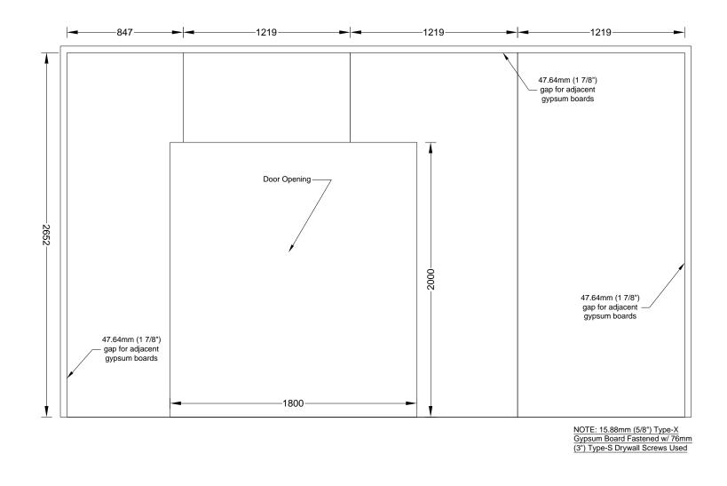
Figure A 17. Test 1-1 Large Compartment CLT - W2 - Gypsum Layout - Face Layer
