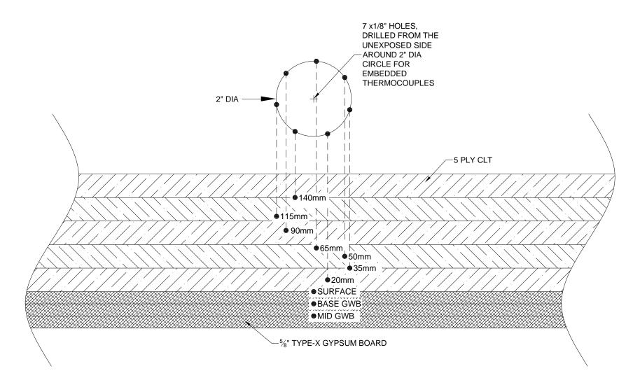
Figure A 65. Test 1-4 Large Compartment CLT - Embedded Thermocouple Detail
