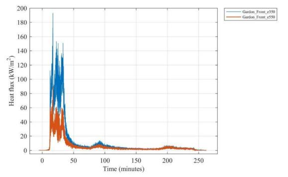
Figure G 15. Heat flux measured by Gardon gauges 350 cm and 550 cm above the floor above the doorway.
