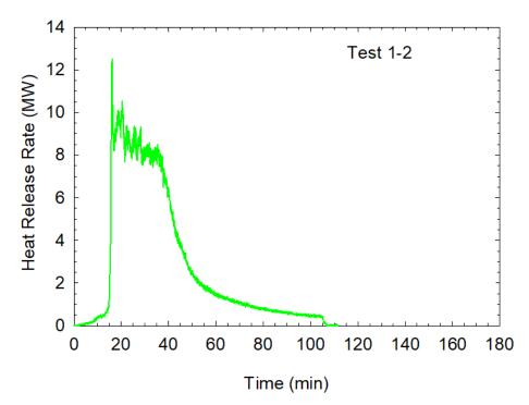
Figure 49. Heat release rate during Test 1-2 (test terminated at 104 min).
