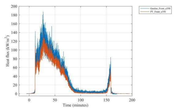
Figure H 21. Comparison of heat fluxes recorded by a collocated Gardon gauge and plate thermometer (PT) 350 cm above the floor above the doorway.
