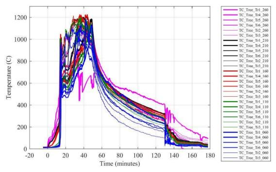
Figure E 8. Thermocouple tree temperatures at various locations inside the compartment.
