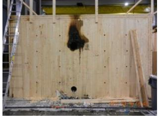
(e) drilled holes through wall panels (f) cutting sample for char measurement Figure 86. Observation and measurement of char after Test 1-5.
