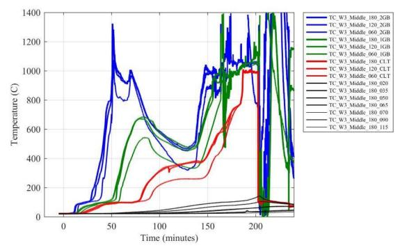
Figure I 12. Temperatures in Wall W3 at various depths from the fire exposed surface.
