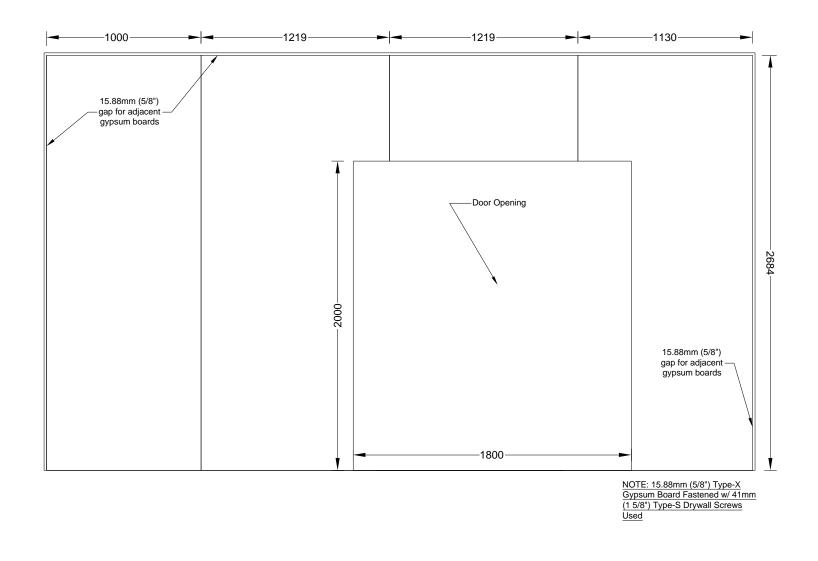
Figure A 72. Test 1-4 Large Compartment CLT - W2 - Gypsum Layout - Base Layer
