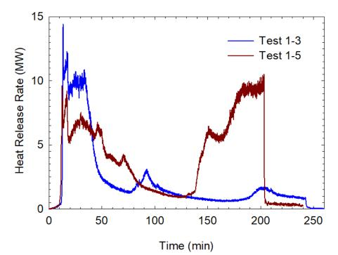
Figure 90. Effect of ventilation – Heat release rates in Test 1-3 and Test 1-5.
