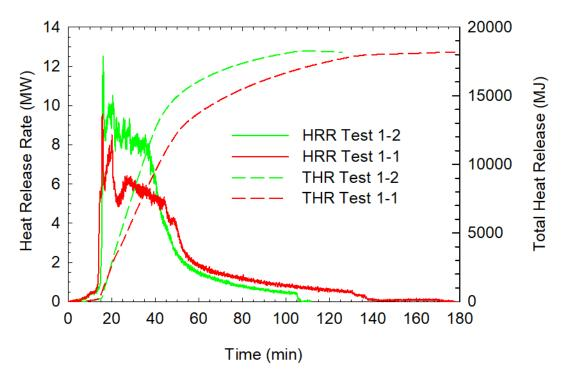
Figure 54. Heat release rates and total heat releases in Test 1-1 and Test 1-2.
