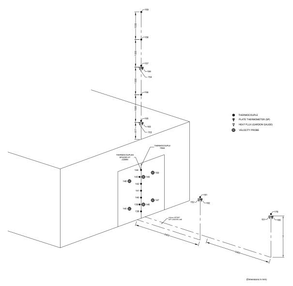
Figure A 68. Test 1-4 Large Compartment CLT - Exterior Instrumentation Layout
