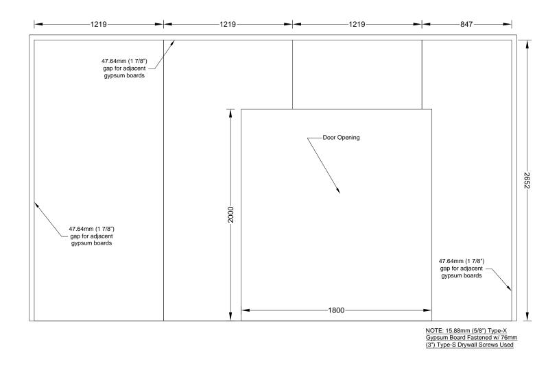
Figure A 56. Test 1-3 Large Compartment CLT - W2 - Gypsum Layout - Face Layer
