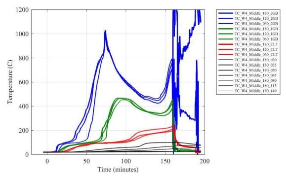
Figure H 13. Temperatures in Wall W4 at various depths from the fire exposed surface.
