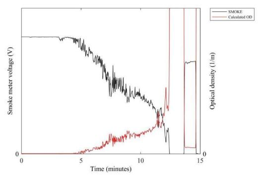
Figure G 25. Smoke meter voltage and calculated optical density (OD) from gas sampled at the center of the compartment 160 cm above the floor.
