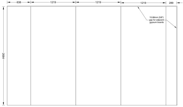
NOTE: 15.88mm (5/8") Type-X Gypsum Board Fastened w/ 41mm (1 5/8") Type-S Drywall Screws Used
