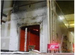
(g) at 122 min (h) at 151 min, second flashover **Figure 72. Photographs of the CLT compartment during Test 1-4.**
