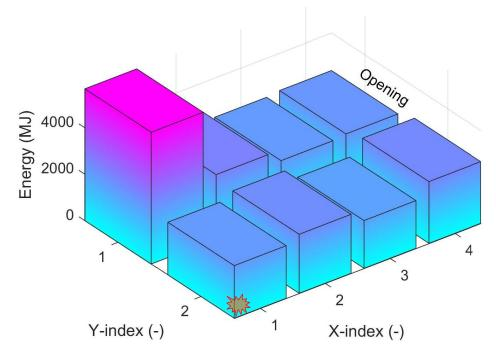
Figure 17. Isometric view of the movable fuel energy as installed (4 × 2 regions).
