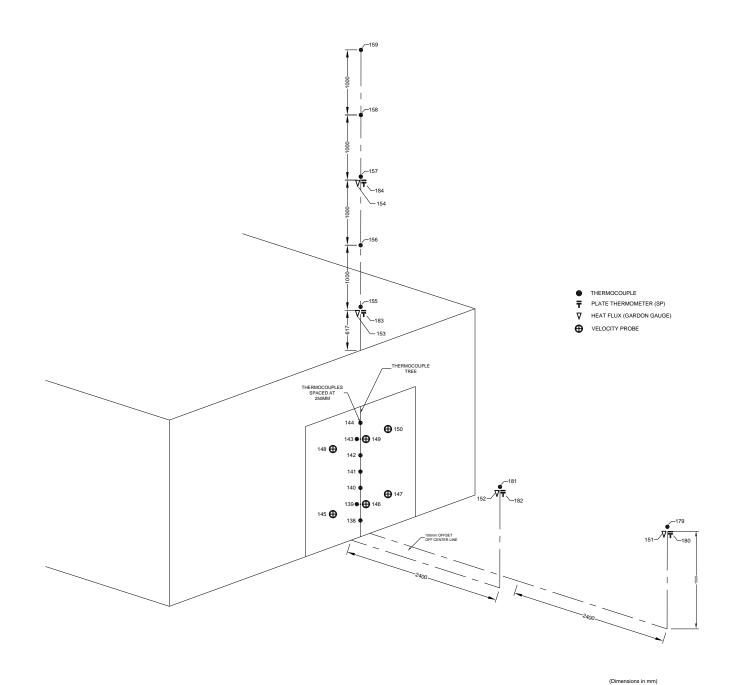
Figure 27. Measurements in the doorway and outside the compartment.
