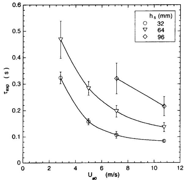
**Fig. 3. Measured characteristic mixing time.**
