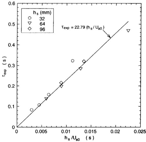
**Fig. 4** Correlation between the characteristic mixing time and the step height normalized by the air velocity.
