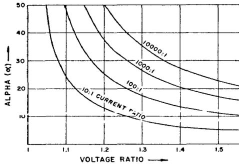
Fig. 6 Clamping ratios for different current ratios as a function of alpha ( $\alpha$ ).
