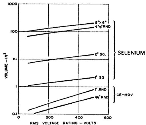
Fig. 20 Suppressor volume requirements.
