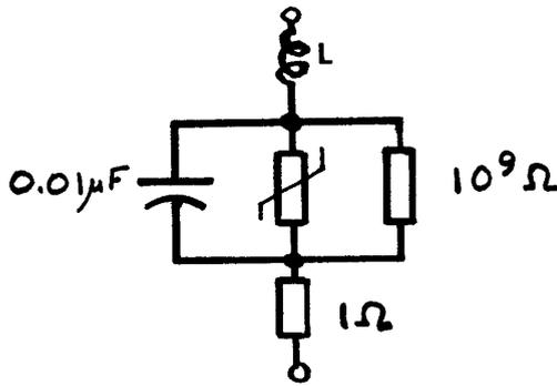
Fig. 8 MOV varistor elementary equivalent circuit.
