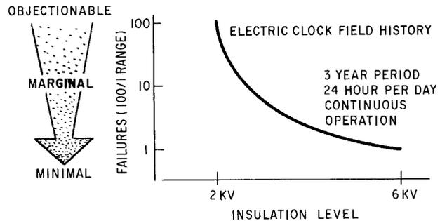
Fig. 11 Electric clock (line operated) field history.
