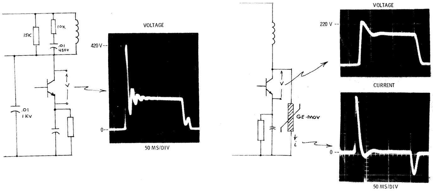
Fig. 18. Application of varistors in A-M receiver.
