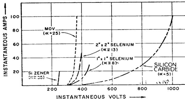
Fig. 24 Linear volt/ampere characteristics of common voltage suppressors.
