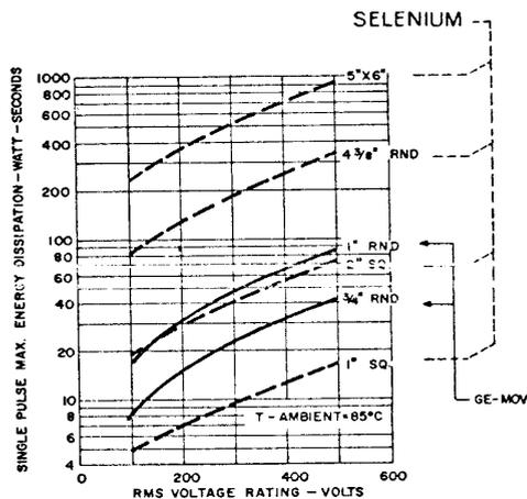
Fig. 22 Suppressor energy dissipation capability.
