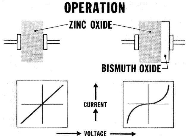
Fig. 3 V-I characteristic of zinc oxide and ZnO-Bi<sub>2</sub>O<sub>3</sub>.
