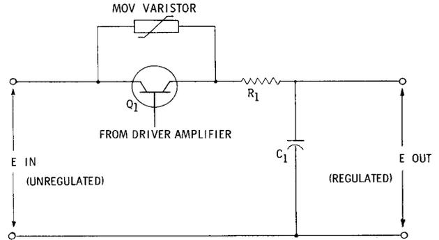
Fig. 17 Start up transient voltage surge protection.
