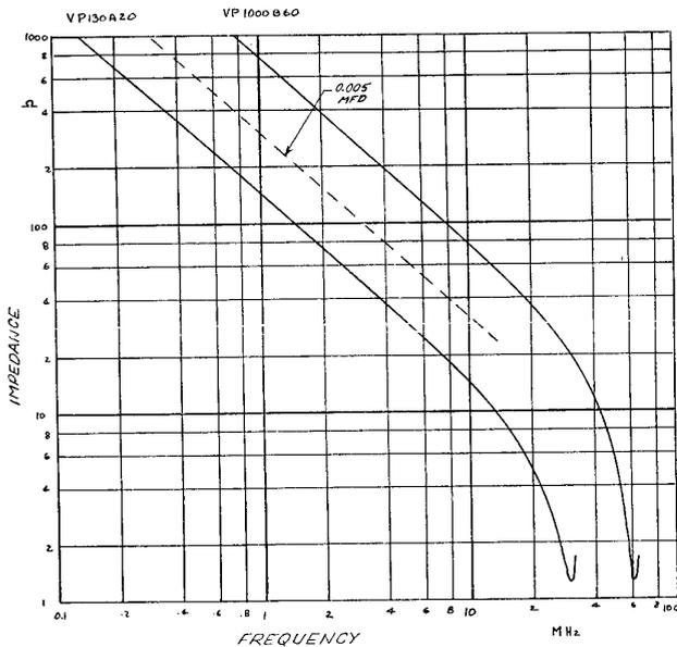
Fig. 10 Typical VP series capacitance.
