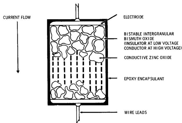
Fig. 1 Structure of metal oxide varistor.
