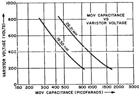
Fig. 9 Typical capacitance.
