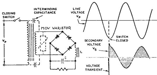
Fig. 16 Voltage transient due to energizing step-down transformers.
