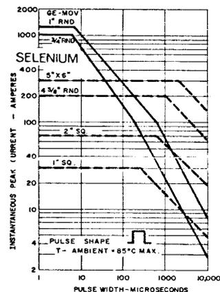
Fig. 21 Suppressor peak current capability.
