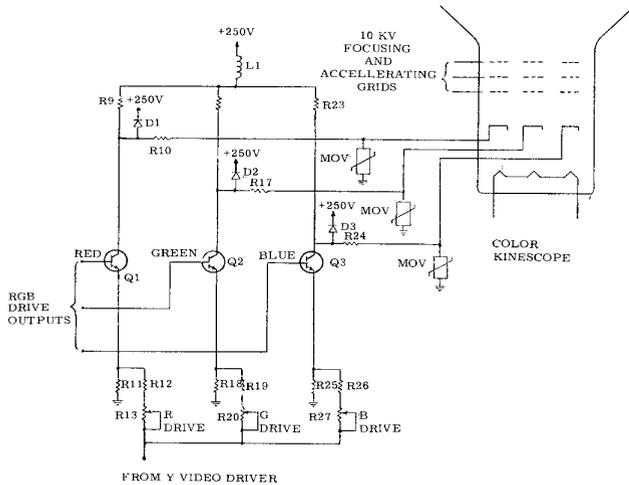
Fig. 19 Color RGB video driver protection from arcing kinescope.
