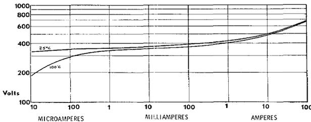
Fig. 7 Typical VP series temperature effect.
