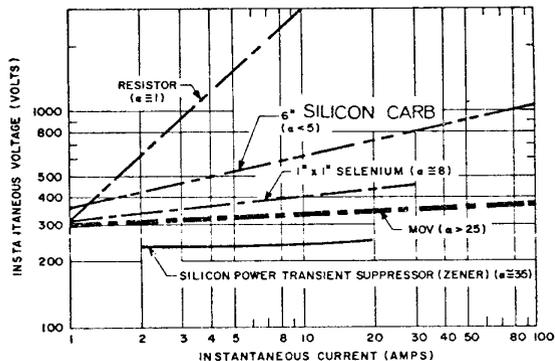
Fig. 23 Log-log volt/amperes characteristics of common voltage suppressors.
