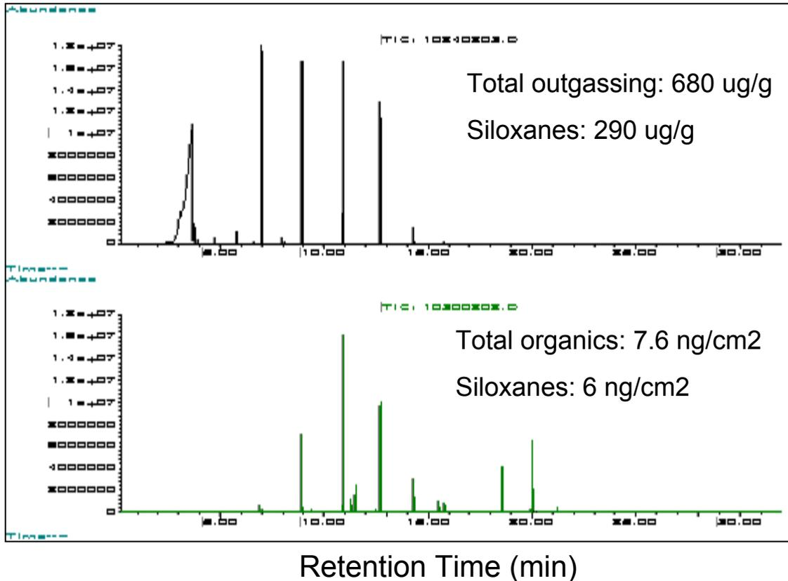
**Direct outgassing of a sealant**
