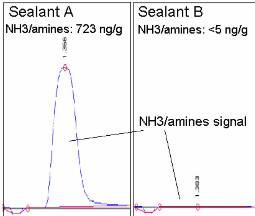
Sealant A caused significant T-topping defects in E0 delay photoresist test due to its high NH3/amine outgassing.
