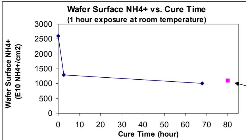
Surface NH<sub>4</sub><sup>+</sup> of witness wafers exposed to same sealant: room temperature
