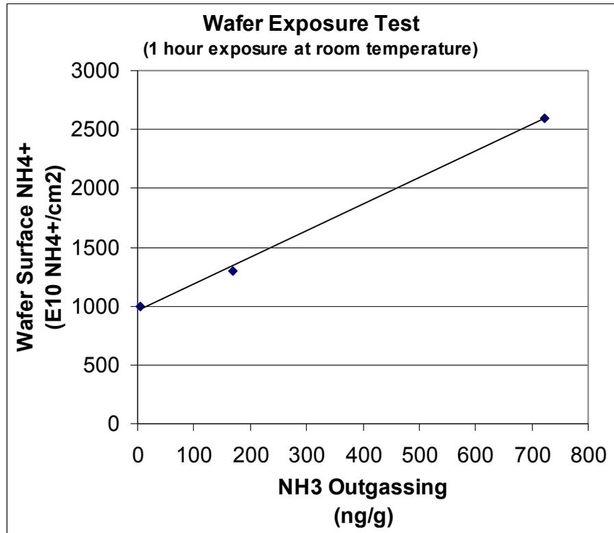
Linear relationship between witness wafer surface NH4+ and sealant NH3/amines' outgassing concentration
