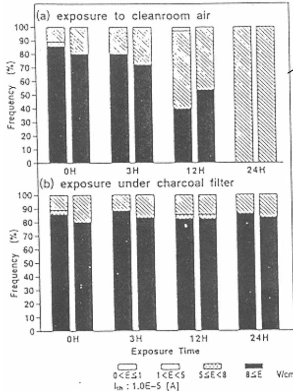
Wafers exposed to cleanroom w/o chemical filters
