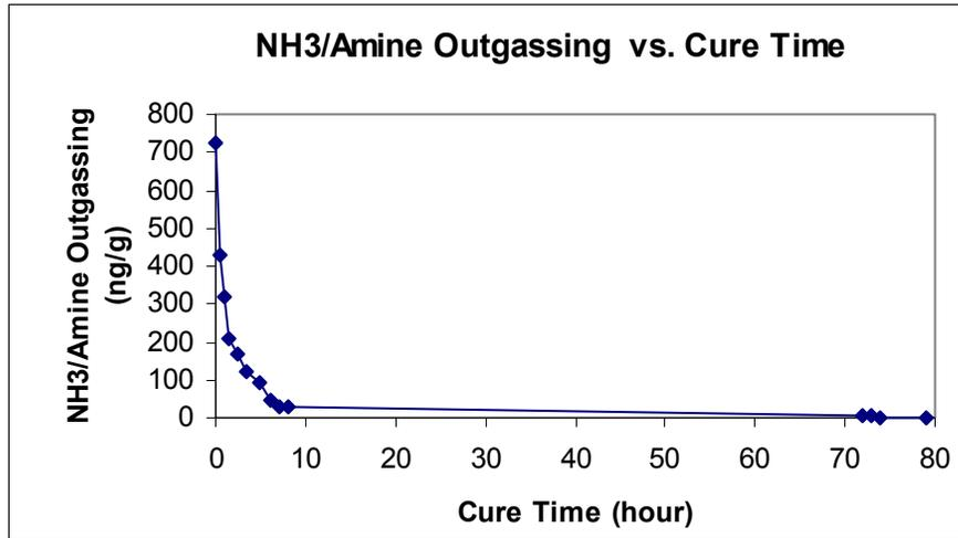
Time dependent NH<sub>3</sub>/amine outgassing of a sealant: room temperature
