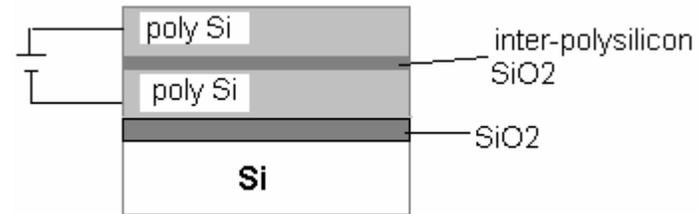
Device structure used to measure breakdown strength of inter-polysilicon SiO2
