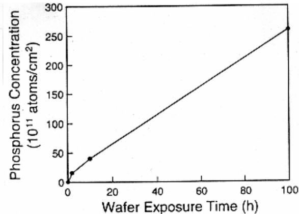
Fig. 4. Phosphorus contamination measured on witness wafers as a function of exposure time to Fab 1 air.
