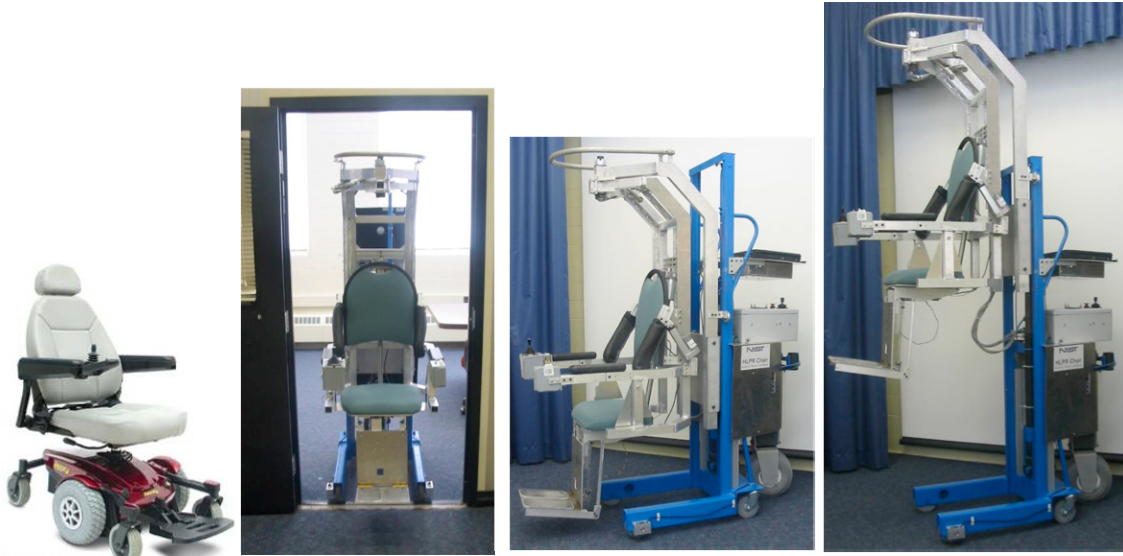
Figure 3: Typical powered chair (left) [courtesy Jazzy 1 ] and the HLPR Chair 1 prototype (right three photos). HLPR Chair is shown in the mobility (center photos) and the lift (right-most) configurations. Note the unique shape of HLPR Chair as compared to typical powered chairs.
