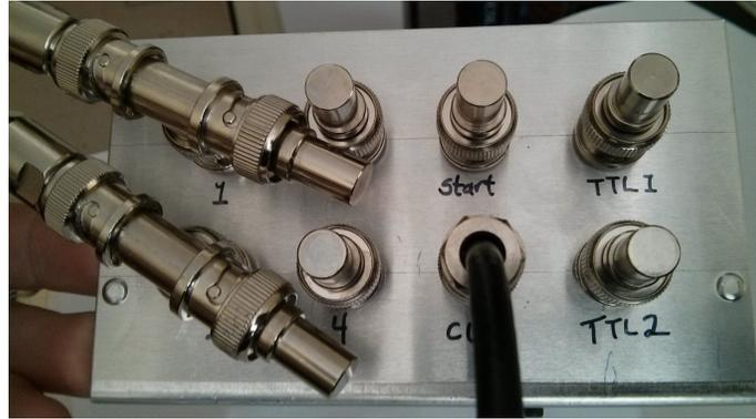
Figure 3: Proper 50  $\Omega$  BNC termination.
