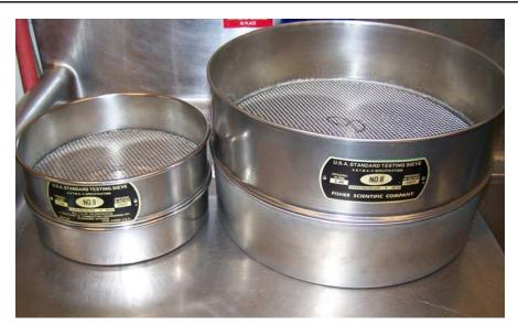
Use a Number 8 mesh sieve: 8" diameter for packages 1 lb or less, 12" diameter for packages over 1 lb.
