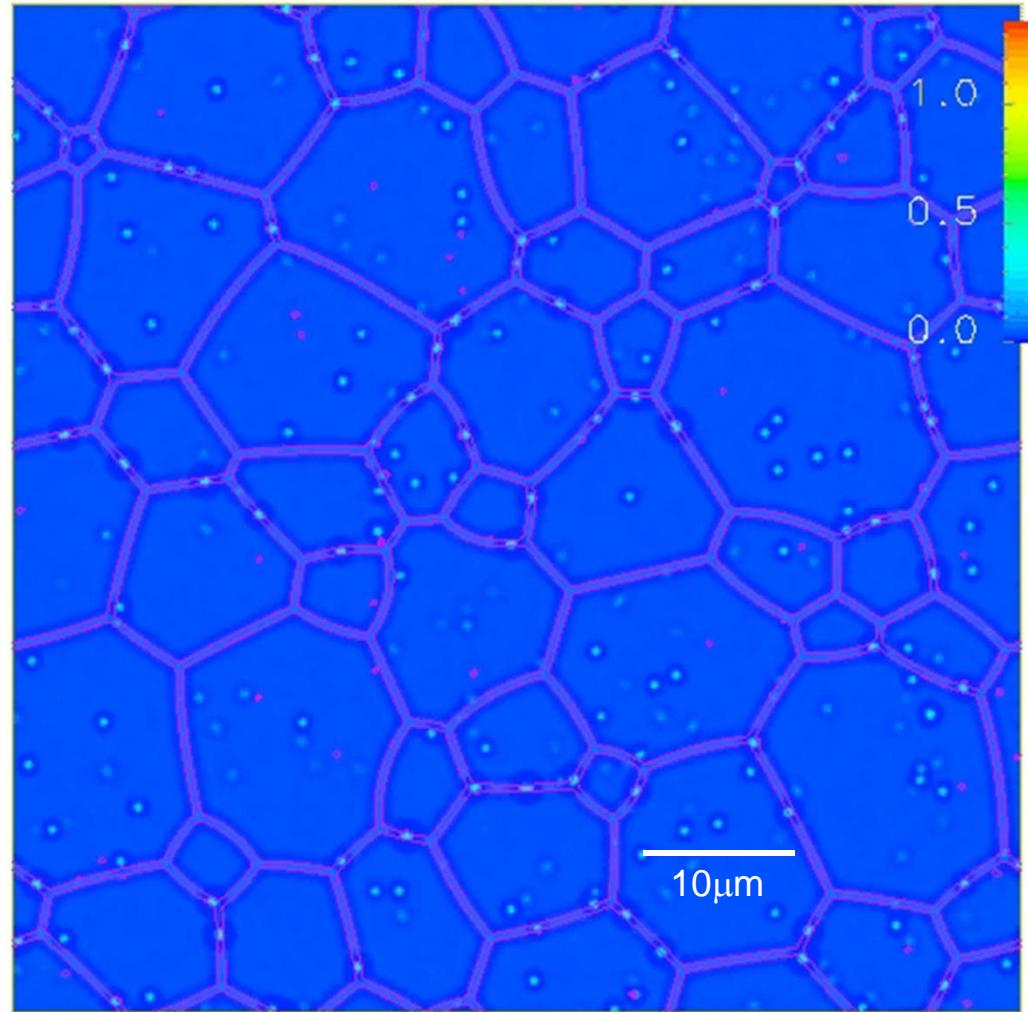
Simulation of gas bubbles evolution in polycrystalline  $\text{UO}_2$  fuel<sup>1-3</sup>.
