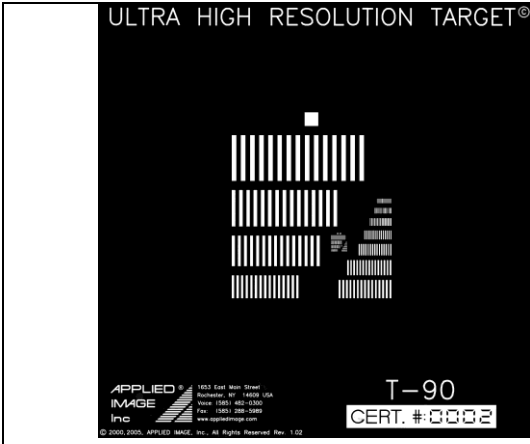
Figure 14. This example uses a transparent T-90 high resolution target printed on clear glass with 3 groups of line pairs. A high resolution target printed with chrome on opal glass will also work.
