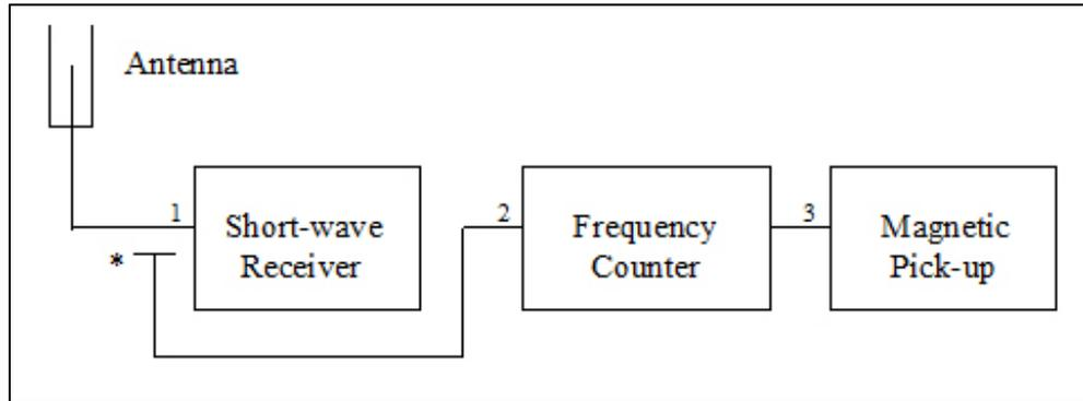
**Figure 1. System Configuration.**
