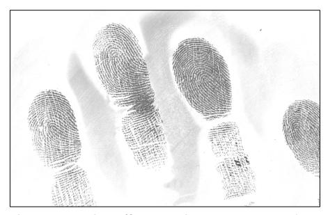
Figure 4. Moisture/Condensation on the platen surface.
