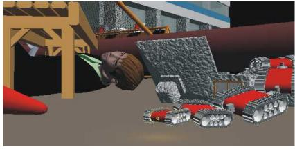
The robot is constructed by caterpillar type machines. Machines are connected sireally with active or passive joints.
