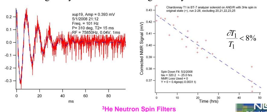
Flipping ratio can also be used to monitor the 3He polarization although it is not straight forward and we do not prefer because it involves in polarization efficiency correction. However, unpolarized neutron transmission measurements are much better.
