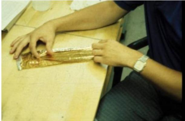
The blocks were wrapped in Mylar, the comparator put in a insulated box with face shield, and the operator wore a cape, big gloves, and worked quickly.
