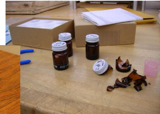
Most cases are designed to protect the gages in the lab, not for shipping. On the left, the box has allowed a high stakes billiards game with precision gages. Wires, on the other hand, are in separate tubes.
