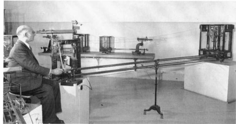
Plate 34: Albert Bonhoure operating the Ruprecht No.1 balance in Room 5 of the Observatoire, date unknown but probably in the 1940s or 1950s; all balances were operated at a distance to avoid heating by close proximity of the operator. (Courtesy BIPM.)
