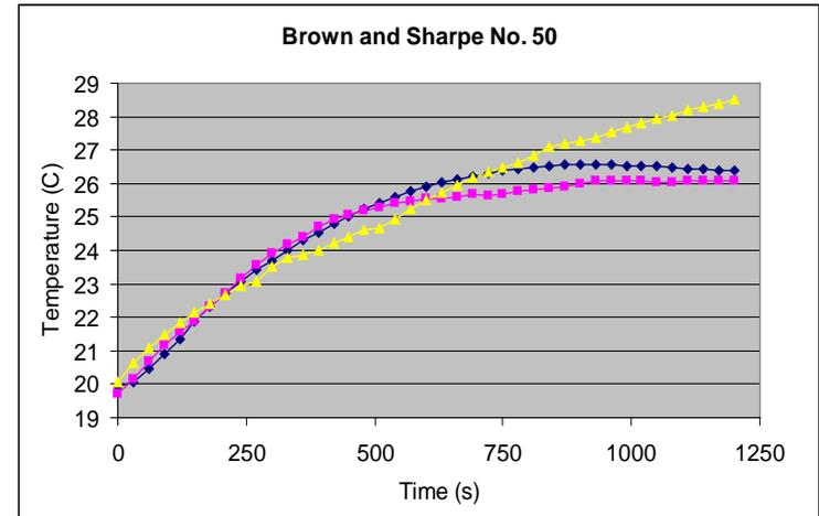
Using a thermal expansion coefficient of 12 PPM/°C and the fact that the maximum range of the Brown and Sharpe #50 micrometer is two inches, the error in measurement caused by a shift of 6 °C is 3.07  $\mu\text{m}$ . The same test with a micrometer with a thermal insulating plate reduced the effect considerably.
