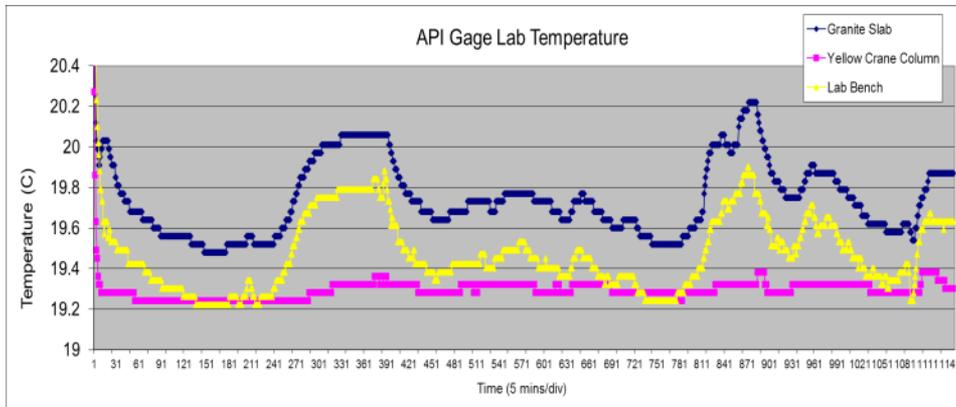
In our conventional labs, where the temperature is controlled to about 0.5 °C we see temperature differences of about that size. Large machines have a large thermal mass, effectively filtering the temperature changes..
