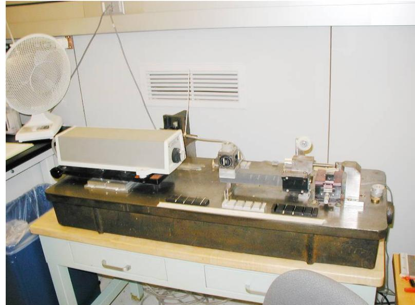
This is our holder for balls and wires. The “V” grooves have cone do not provide as much thermal conduction as gage blocks on a plate, but these are generally small gages with little thermal mass.
