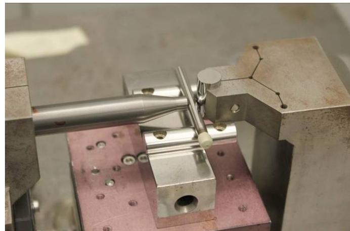
For small cylinders supported by two parallel half-rounds, the micrometer force will align the gage surface to the micrometer contact. As the cylinders get bigger, static friction becomes greater and alignment errors are common.
