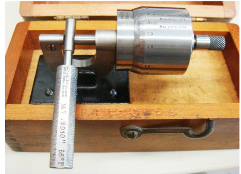
If the scale is directly on the measurement line the effects of pitch errors in the instrument are greatly reduced or eliminated. Note that a micrometer has its scale (lead screw) aligned with the center of the contacts.
