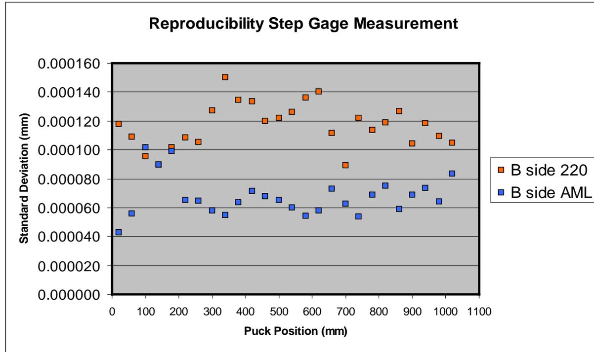
This shows the history of our 1020 KOBA run on the same machine, the Moore M48. The top data is the old  $\pm 0.1$  °C laboratory. The bottom data is from the AML with its  $\pm 0.01$  °C laboratory. The difference is dramatic, lowering our uncertainty by 50%.
