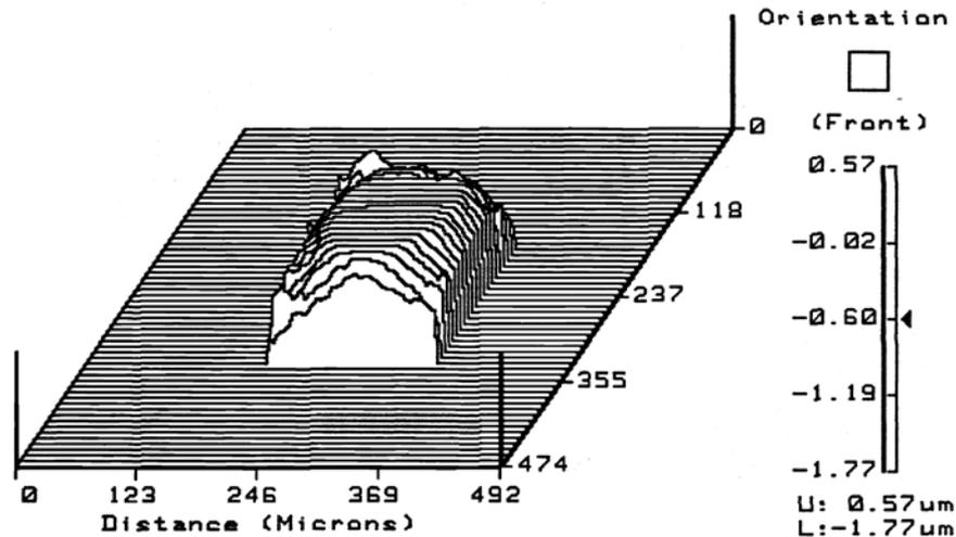
We also assume we know the geometry of the contact. This is the surface of one diamond contact on our gage block comparator. It is remarkably flat with a diameter of over 100  $\mu\text{m}$ , reducing the deformation by 30 nm. This is larger than our uncertainty!
