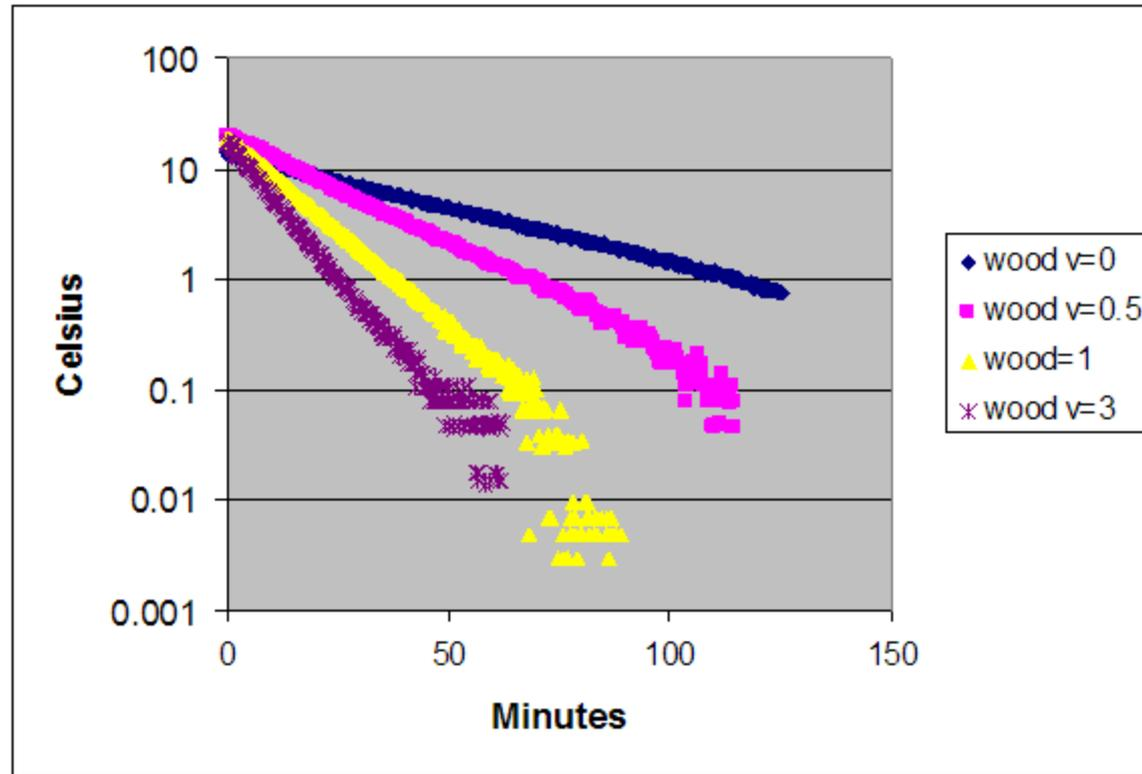
This logarithmic plot shows that the exponential decay model works very well, and the addition of the fan has a dramatic effect.
