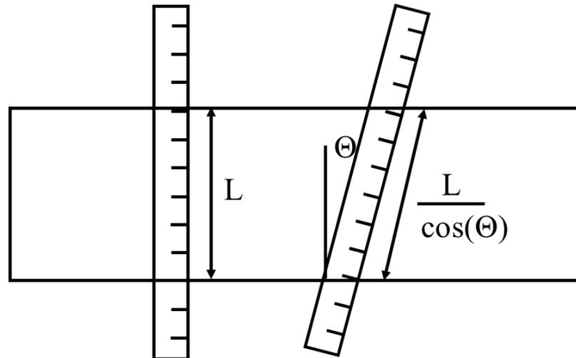
An angle of 5' will produce an error of 1 ppm. This is generally not a problem with modern instruments..
