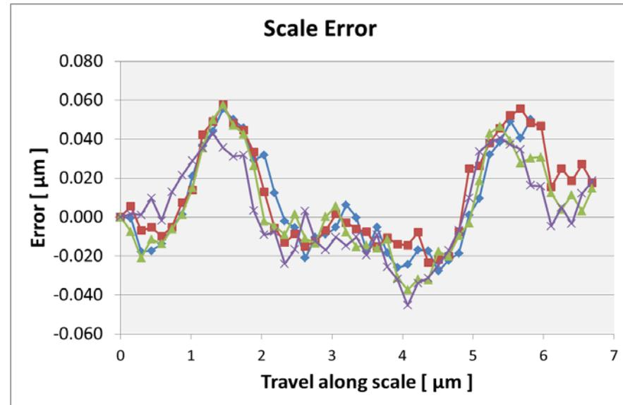
The graph on the left shows a typical response, it is from a Heidenhain Brochure, and it is about 1% of the pitch. On the right is the error measured on a measuring machine in my lab. Our machine has 4  $\mu\text{m}$  pitch so the error should be about 40nm, and it is.
