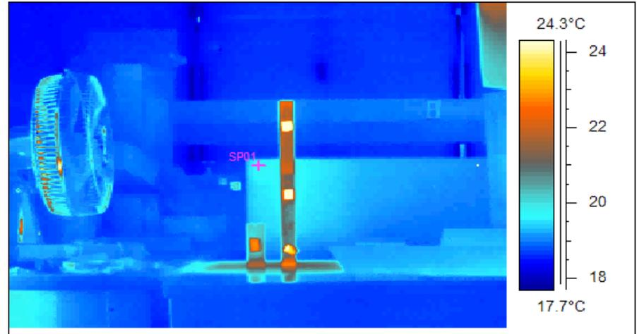
Each of the 500 mm gage blocks have three strips of tape as the thermometry target. The fan can be seen in the background and the anemometer extends horizontally from the right side of the picture.
