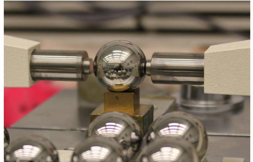
Balls need one degree of freedom so the micrometer can push them till contact. Generally this is a tiny V-block.
