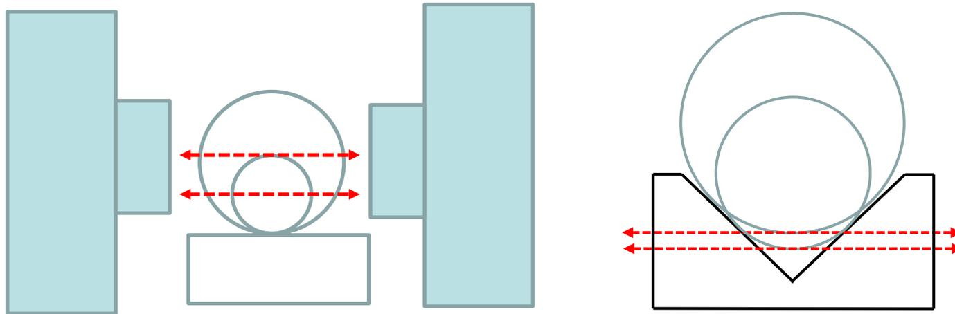
Here we see two balls held up by the same table, and the two spheres contact different places on the anvils. This adds the flatness and parallelism of the contacts to the error budget.
