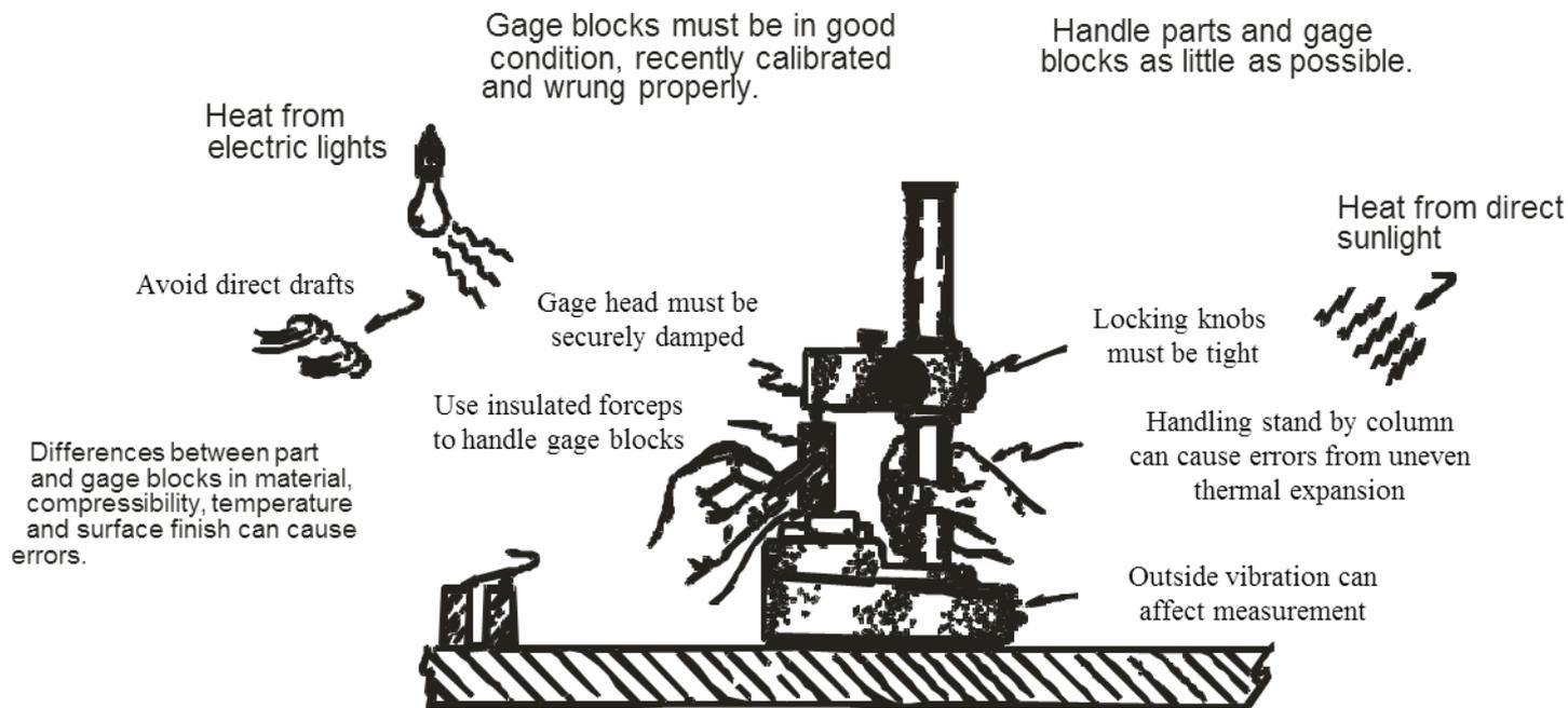
Figure 11-37. All sources of potential errors should be consciously investigated whenever a high precision measurement is made.
