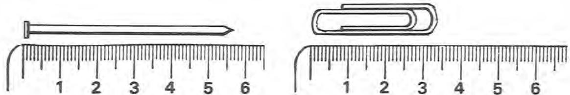
Look at the picture of the nail next to the ruler. The nail is 57 mm long. This is 5 cm + 7 mm. There are 10 mm in each cm, so 1 mm = 0.1 cm (one-tenth of a centimetre). This means that 7 mm = 0.7 cm, so 57 mm = 5 cm + 7 mm
