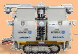
High pressure water injection platform truck
