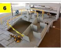
Small scale versions of the standards (6) help inspire confined space capabilities and emerging 3D printed robots. These mini-arenas are used by STEM robot competitions to guide development and measure progress in 3D printed robot designs.
