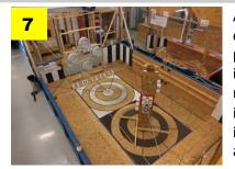
Aerial test methods (7) will enable users to evaluate airworthiness and safety, guide purchases, and help operators measure and improve their proficiency before flying in the national airspace. All testing is conducted indoors or in tents when GPS functionality is involved. Similar tests are being developed for aquatic vehicles within a water tank (8).
