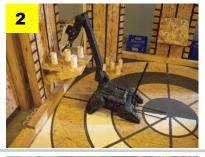
Many of the standard test methods are useful as training tasks. The suites of basic dexterity tasks (2), terrains, and obstacles (3) are particularly useful as repeatable tasks. Any operator can compare their rate of performance to that of the "expert" provided by the robot developer.
