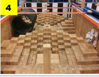
Application specific test methods leverage, extend, or combine, apparatuses to form more complex tasks. Advanced mobility terrains (4) affect performance of all tasks contained within. In another example, vehicle—borne improvised explosive device tasks (5) require dexterity with extended reach and strength in confined spaces.
