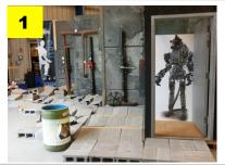
The DARPA Robotics Challenge (DRC) theme focused on emergency tasks at nuclear facilities (1). Reconfigurable terrain complexity challenges basic dexterity tasks such as inspect, touch, rotate, and extract. This approach also works for valves at various elevations and orientations. These were just a few of the 8 test methods used to evaluate international teams at the DRC.
