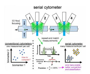
Serial cytometry involves making repeated measurements of single objects as they pass through multiple interrogation regions in a microfluidic channel. Integrated optical waveguides deliver and collect light from objects. Matching and analysis of signals from individual cells, for example, enable uncertainty estimates on the biomarker content of each cell, which enables better comparison and classification of cells and mixture of cells.
