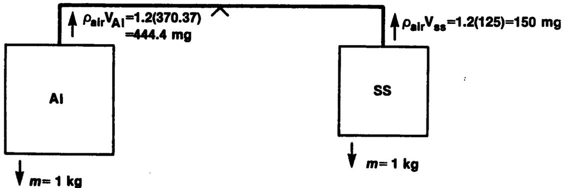
The aluminum weight experiences a much larger lifting effect than the stainless steel weight, namely, 444.4 mg versus 150 mg. Thus, the aluminum weight appears to be 294.4 mg lighter than the stainless steel weight. This is simply the air density times the difference in weight volumes. Hence, the apparent mass of the aluminum weight versus  $8.0 \text{ g/cm}^3$  is approximately
