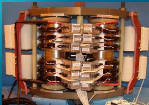
Si 8 kV Clamped Whole Wafer
