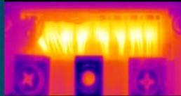
Near-perfect SiC MOSFET Current Sharing In 1200 V / 400 A Module Operating at  $100^\circ\text{C}$  Heat Sink
