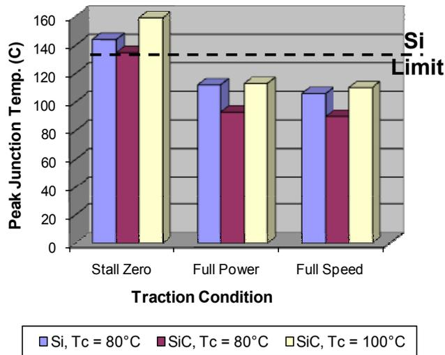
Results from 200-hr Evaluation for 250 kW Traction Drive Application
