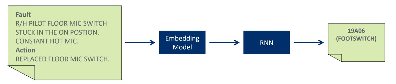
Fault & Action text  $\rightarrow$  Maintenance code Free form text  $\rightarrow$  Malfunction code Maintenance data  $\rightarrow$  Machine summary etc
