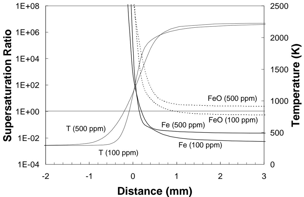
**Fig. 7: Calculated supersaturation ratios ( $S_i = X_i / X_{i,sat}$ ) for Fe (solid lines) and FeO (dashed lines) in a  $\phi = 1.0$  and  $X_{O_2,ox} = 0.21$  flame at  $Fe(CO)_5$  concentrations of 100 ppm and 500 ppm. Note the horizontal line at  $S=1.0$  to mark the saturation point (but not necessarily the condensation point). Temperature profiles are also shown. The location of zero corresponds to the point of 50%  $CH_4$  consumption.**
