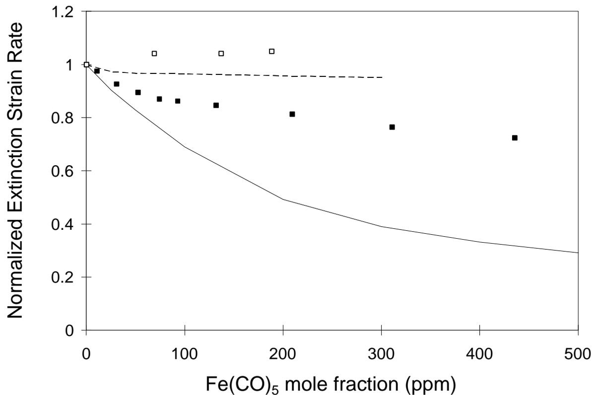
**Fig. 6: Normalized extinction strain rate for counterflow diffusion flame as  $\text{Fe}(\text{CO})_5$  input varies. Closed symbols: measurements with the  $\text{Fe}(\text{CO})_5$  in the oxidizer; open symbols: measurements with  $\text{Fe}(\text{CO})_5$  in the fuel; solid line: calculations with  $\text{Fe}(\text{CO})_5$  in the oxidizer; and dashed line: calculation with  $\text{Fe}(\text{CO})_5$  in the fuel. Experimental data from ref. [6].**
