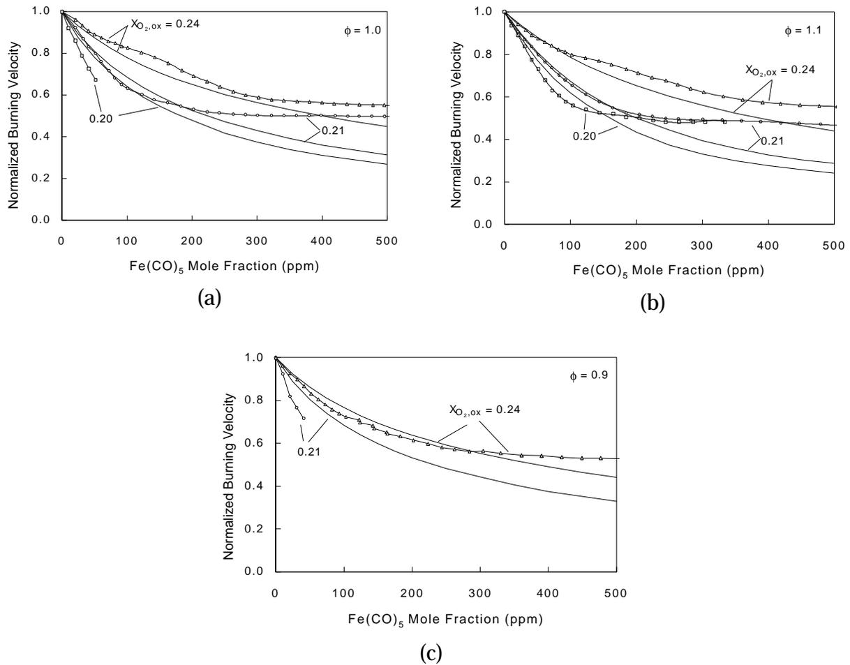
**Fig. 4: Calculations and measurements of normalized burning velocity of premixed  $\text{CH}_4/\text{O}_2/\text{N}_2$  flames with  $X_{\text{O}_2,ox} = 0.20$  (squares),  $0.21$  (circles), and  $0.24$  (triangles). (a)  $\phi = 1.0$ , (b)  $\phi=1.1$ , and (c)  $\phi=0.9$ . Experimental data from ref. [6].**
