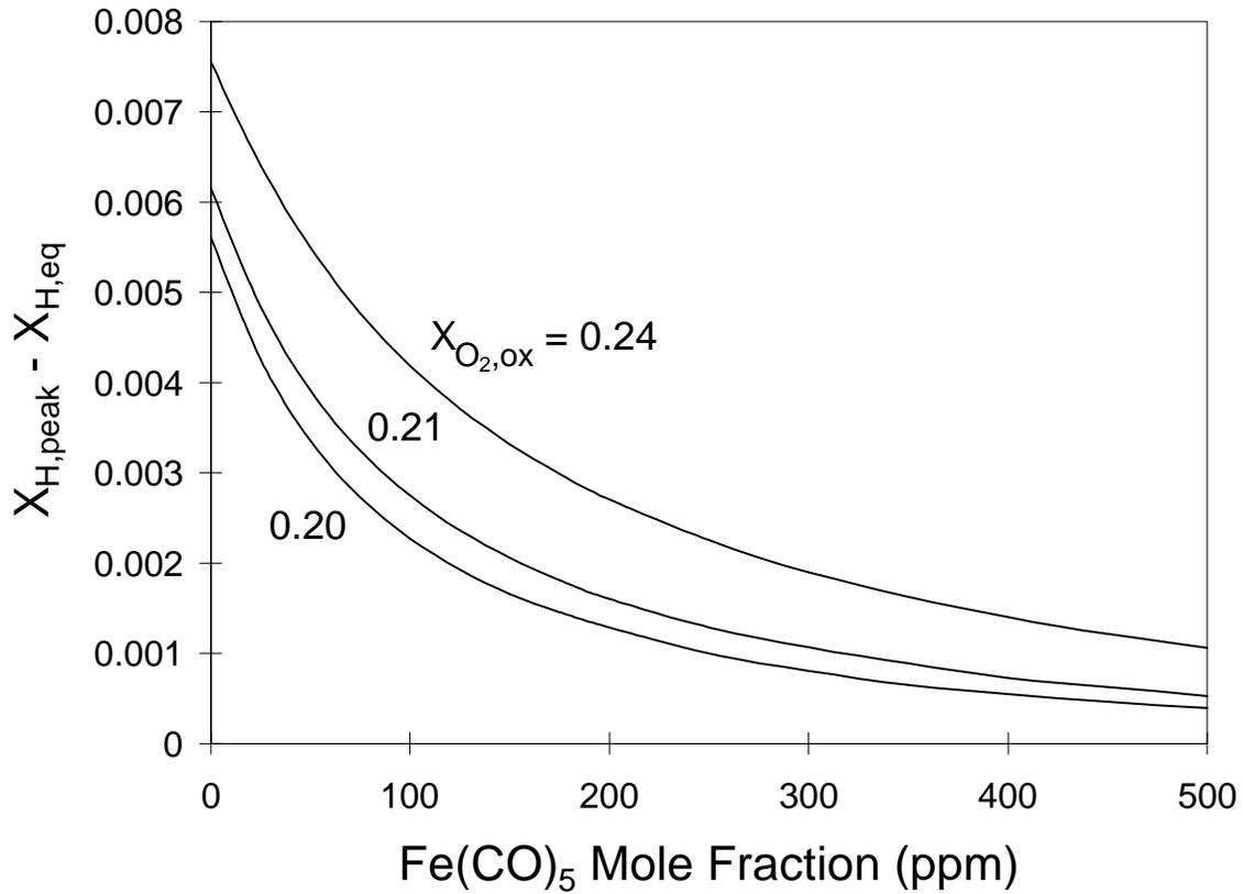
**Fig. 3: Calculated dependence of superequilibrium H-atom mole fraction ( $X_{H,peak} - X_{H,eq}$ ) on  $\text{Fe}(\text{CO})_5$  addition in premixed stoichiometric flames with  $X_{O_2,ox} = 0.20, 0.21,$  and  $0.24$ . The calculated value of  $X_{H,eq}$  is approximately  $2.8 \cdot 10^{-4}$  for  $X_{O_2,ox} = 0.20$ ,  $4.1 \cdot 10^{-4}$  for  $X_{O_2,ox} = 0.21$ , and  $1.0 \cdot 10^{-3}$  for  $X_{O_2,ox} = 0.24$ .**
