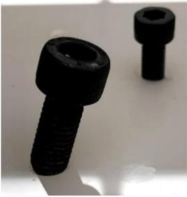
Cross threaded screw cannot advance thread by hand (no points)
