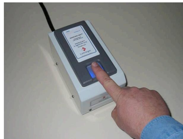
Prototype of Lumidigm / Cross Match two-camera sensor
