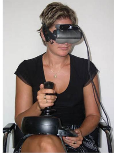
*Figure 8: Orpheus control with joystick and head mounted display*
