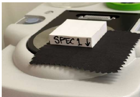
Figure 1: Example of single layer of fabric with 99 % reflectance calibration target. Here, the detector is below the fabric, so the calibration target is placed on top of the fabric.
