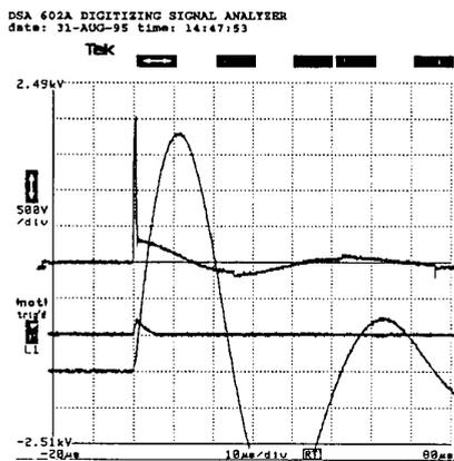
**Figure 8 - Voltages and currents with gap set to sparkover at 2 kV**
