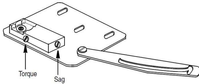
**Figure 1.** Undercounter Hinge Bracket for Glass Door Adjustments
