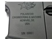
Laser engraved serial numbers are difficult to restore. EBSD can detect changes in the material structure induced by the laser.
