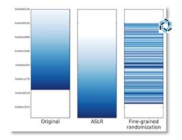
exploitation by varying the attack surface (the layout of your code, see figure). This entropy makes writing reliable exploits extremely difficult for hackers.
