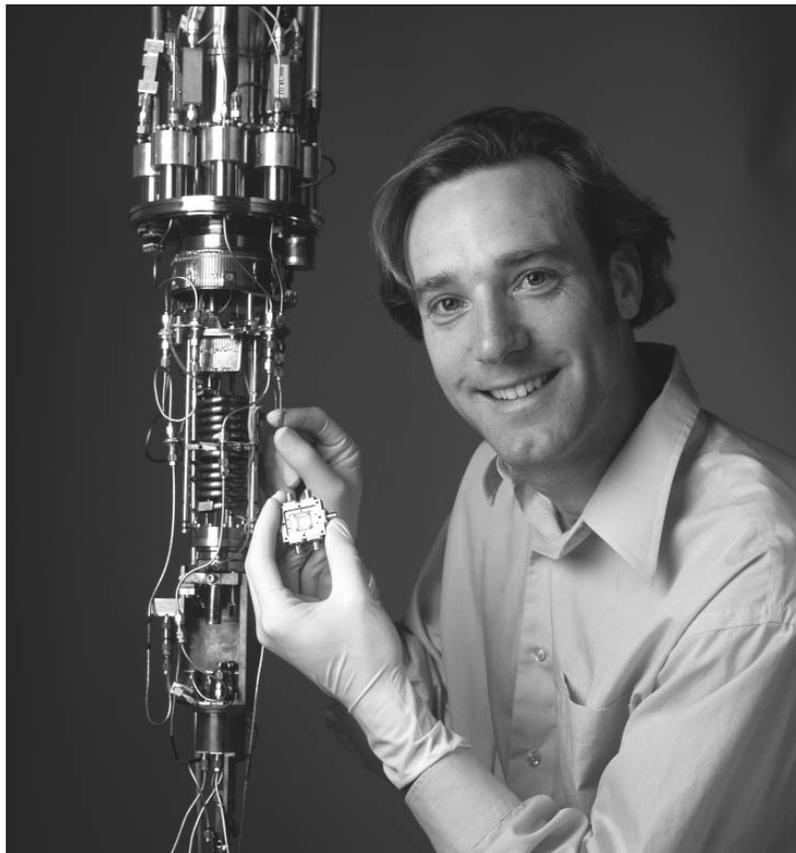
*NIST physicist Ray Simmonds holds a protective box containing “artificial atoms” that might be used in quantum computers. Next to him is a cryogenic refrigerator that cools the box to temperatures near absolute zero.*
