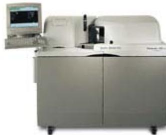
The Dimension, Dade Behring's product line of integrated chemistry systems, provides automated testing techniques for small labs with low-to medium-volume testing. The system offers reagent management to support calibration procedures for routine chemistries. The company offers this type of testing equipment in a variety of sizes tailored specifically to the need for different volumes of testing.
