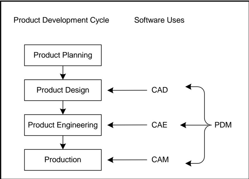
creates a computer image of a two-dimensional or three-dimensional design using a light pen, mouse, or tablet connected to a workstation or personal computer. The design can be easily modified. It can be viewed on a high-quality graphics monitor from any angle and at various levels of detail, allowing the user to readily explore its physical features. Designers can use CAD software to integrate drawings in such a way that adjusting one component alters every attached component as necessary.
