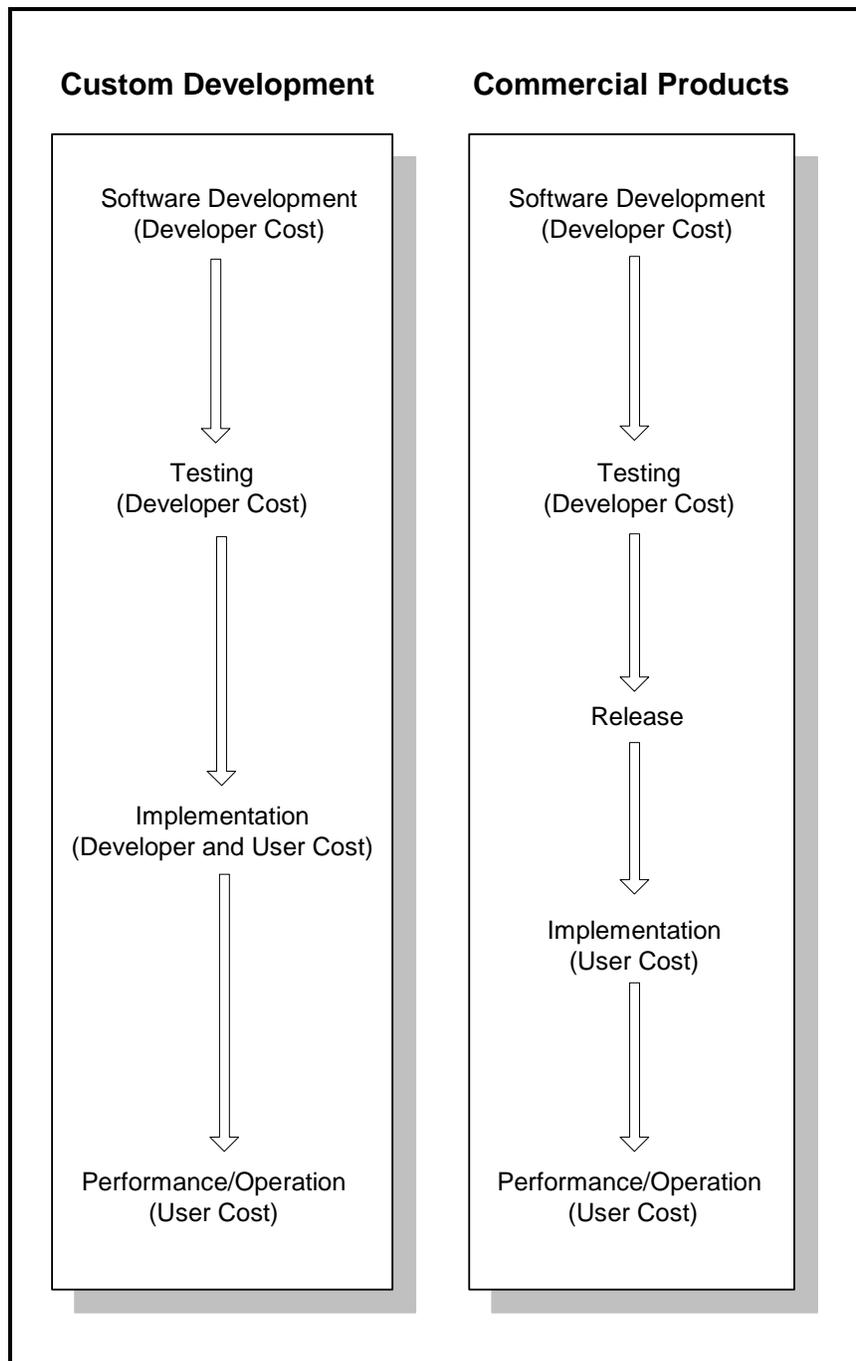
Both custom and commercial (prepackaged) software products have similar production processes. As shown in Figure 5-5, they both start with software design and coding, move to software unit and integration testing, then implementation, and finally to operation and product support.
