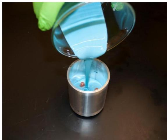
Pouring silicone into replication rig
