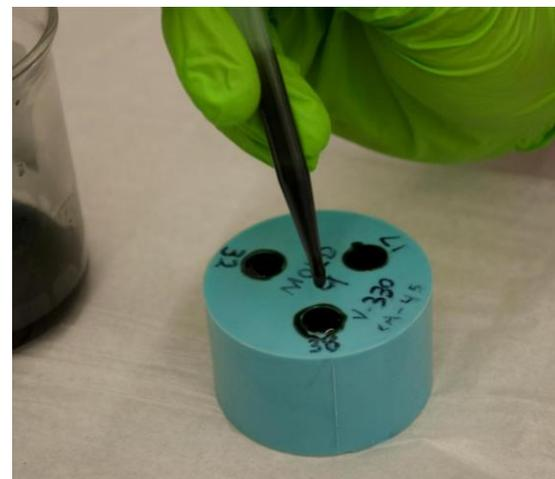
Use a dropper to fill mold with polyurethane. Vacuum-degas again and let cure.
