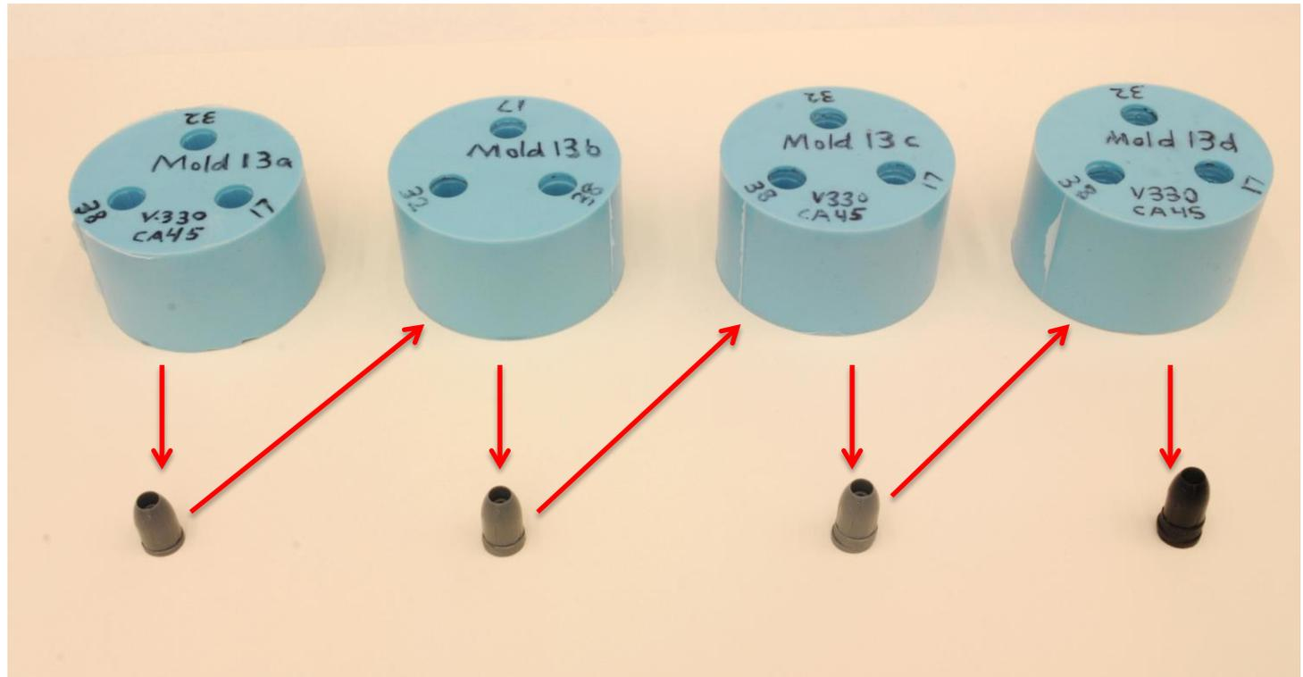
Master Bullet #'s 17, 32, & 38 used to create first mold (13a)
