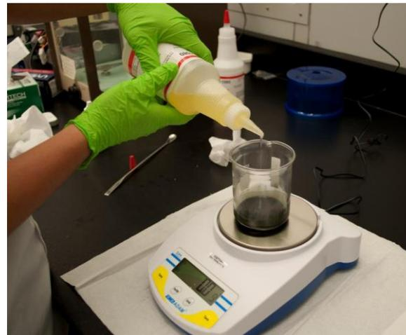
Mix two-part polyurethane and coloring dye. Then vacuum-degas.
