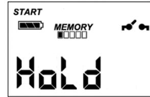
**Image2:** Screen display when button is pushed
