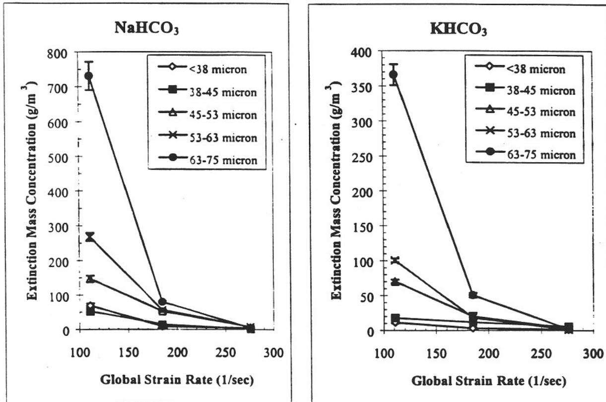
Figure 1: Extinction mass concentration vs. global strain rate as a function of particle diameter for  $\text{NaHCO}_3$  and  $\text{KHCO}_3$ .
