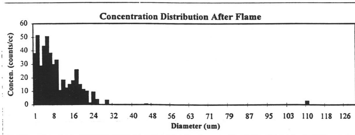
Figure 2: Behavior of Purple-K Commercial Powder at Three Different Axial Positions with Respect to the Flame.
