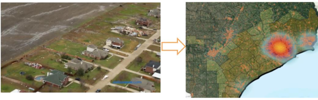
We have developed an automatic damage assessment system using aerial videos from social media or public safety personnel. As shown in the above figure, we aim to build a system that accurately detects buildings and the level of damage in order to help yield faster disaster relief efforts.
