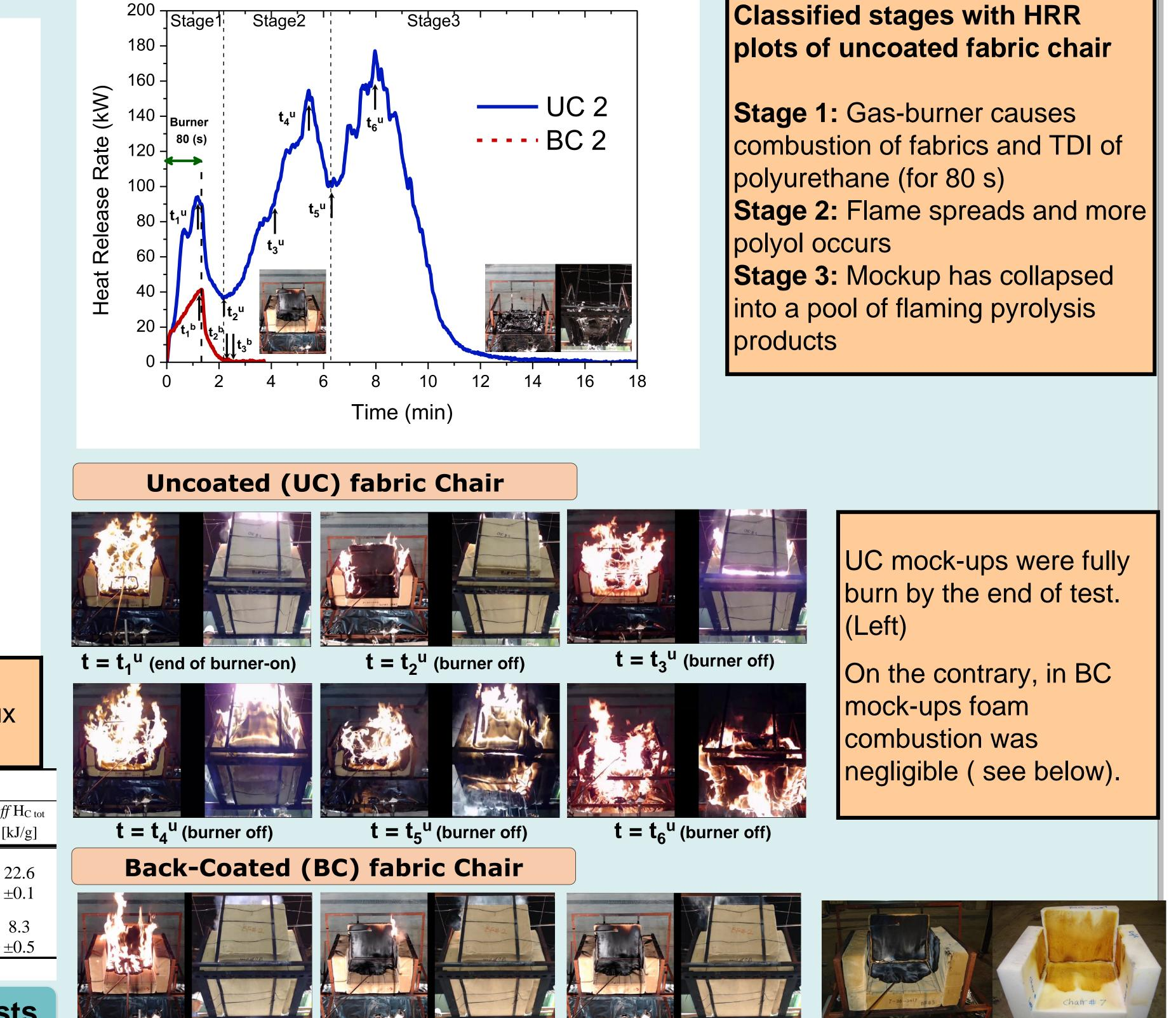
BC technology results in extraordinary reduction of flammability. BC chairs have PHRR and THR as low as 13.5 % and 2.2 % of UC chairs, respectively. Heat flux values up to about 70 kW/m<sup>2</sup> are measured.
