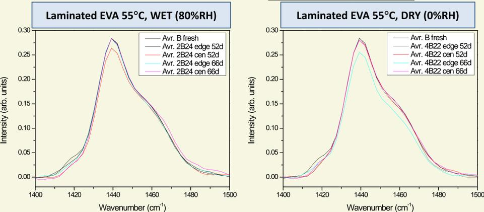
Laminated EVA samples under both WET and DRY conditions indicated a reduction in the crystallinity.
