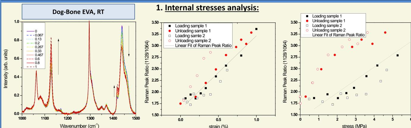
EVA DB samples were strained in steps while continuously monitoring both the load response and the intensity of Raman shift, and a correlation was made. It was shown that the EVA stress and strain can be measured in a non-destructive manner using Raman spectroscopy and it is directly related to the C-C<sub>sym.</sub>/C-C<sub>asym.</sub> stretching.
