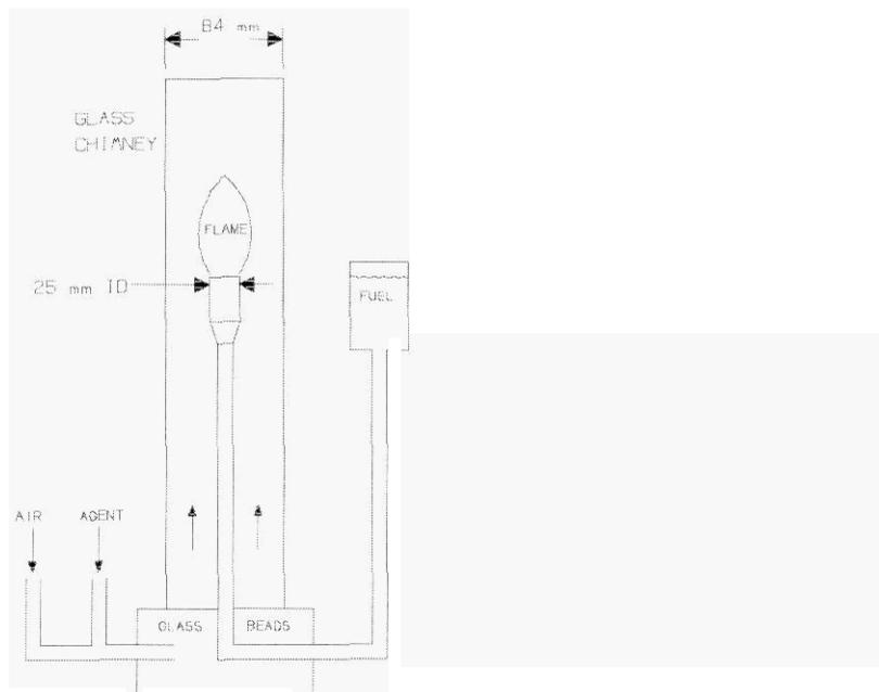
Figure 2. Schematics of the cup-burner assembly.
