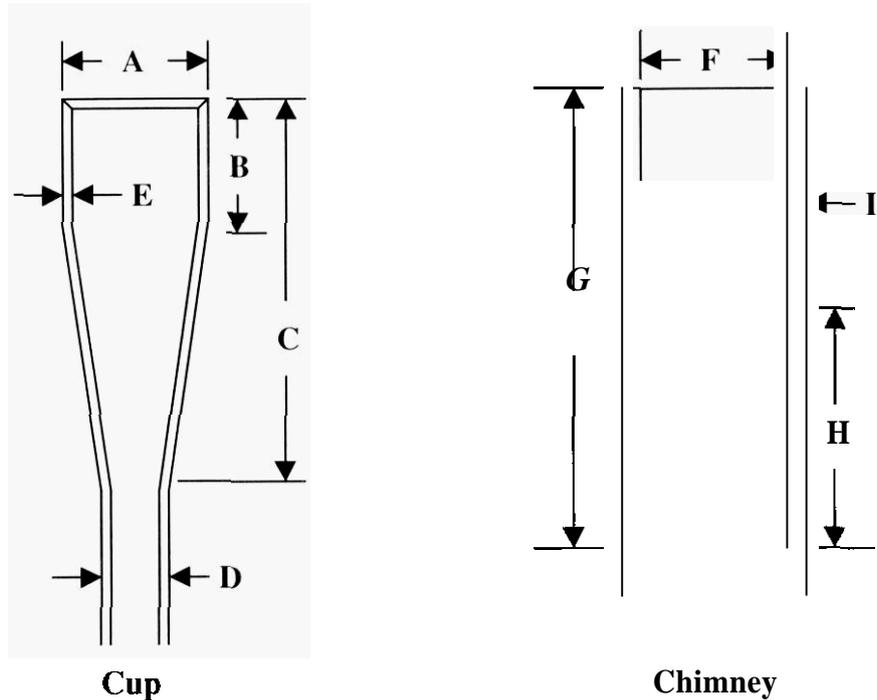
Figure 1. Nomenclature for the **key** dimensions of the cup-burner apparatus.
