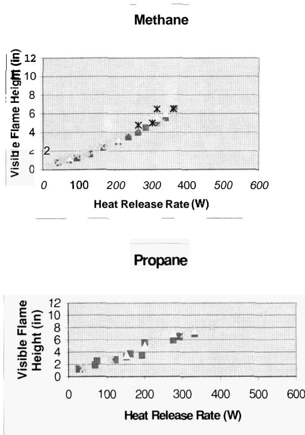
Figure 3. Recorded visible heights for methane and propane flames. Different symbols denote measurements taken by two different operators.
