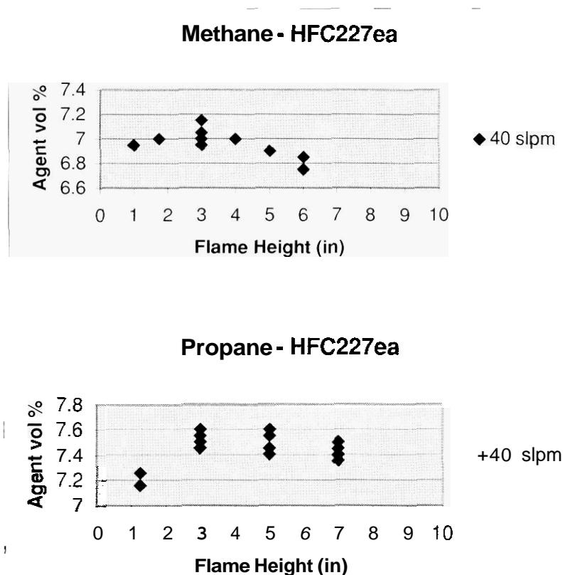
Figure 6. Effect of initial flame height on the extinguishing concentration. Note: A flame that is initially 3 to 4 in tall is most difficult to extinguish.
