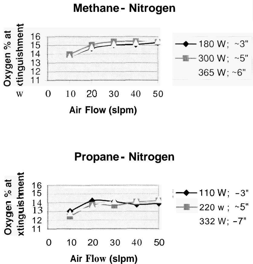
Figure 4. Effect of air flow rate on extinguishing concentration. Each point represents a single test (no repeats).
