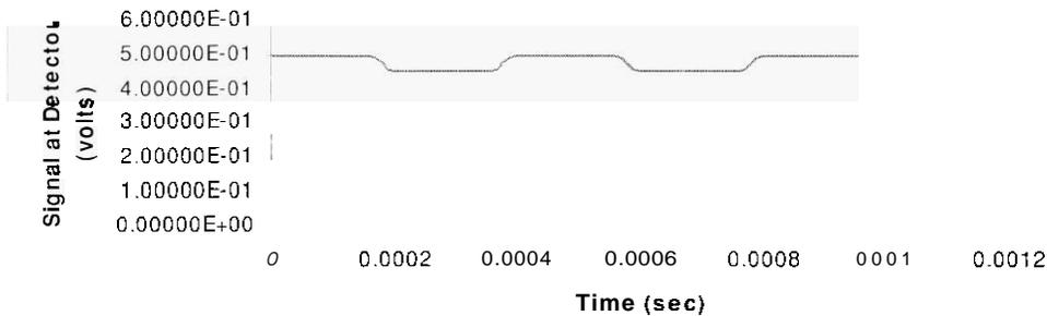
Figure 2. The calculated signal at the detector for a moderately strong absorbing **gas** for square wave modulation of the probe laser beam components.
