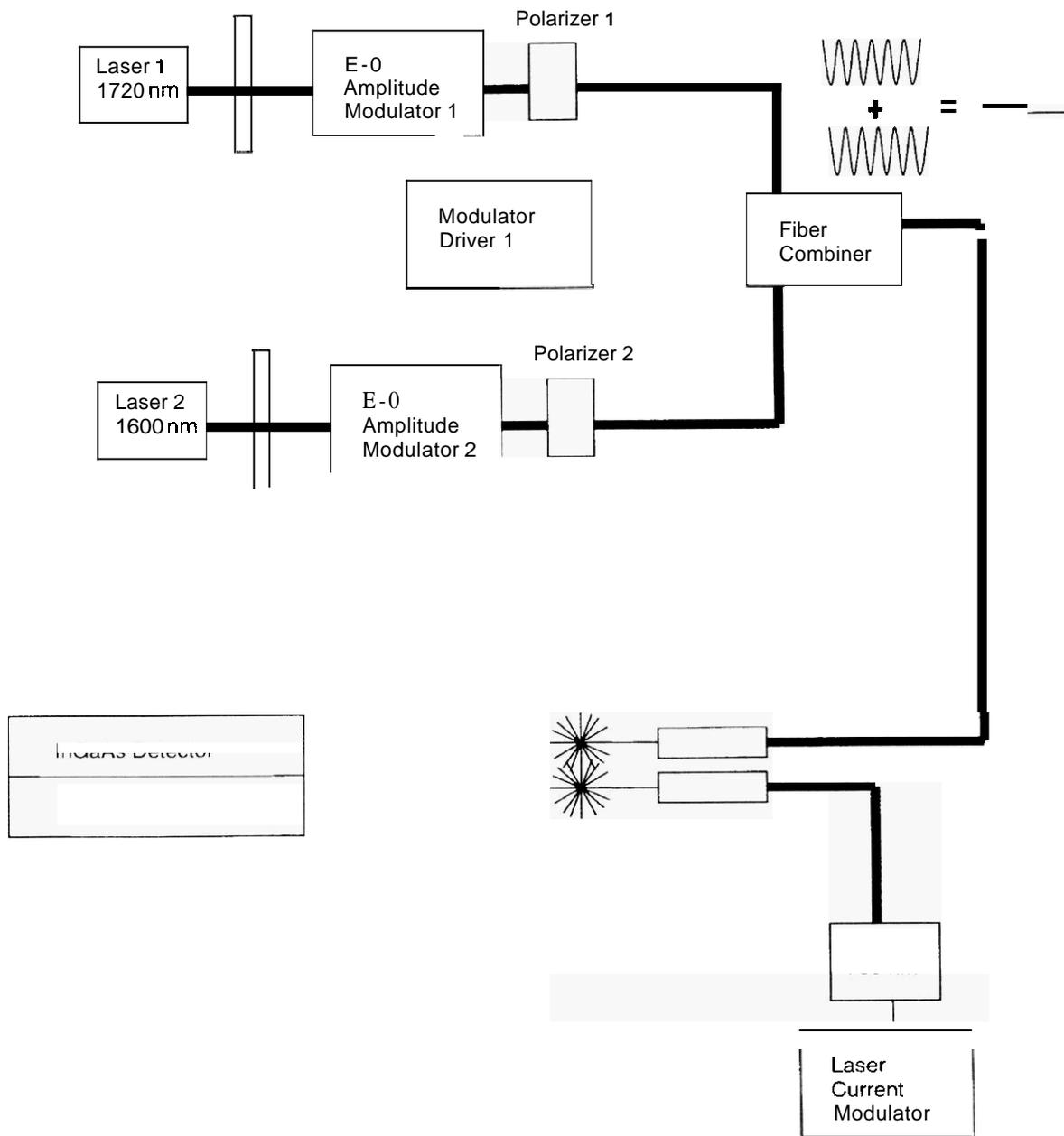
Figure 5. Optical layout of the binary gas sensor
