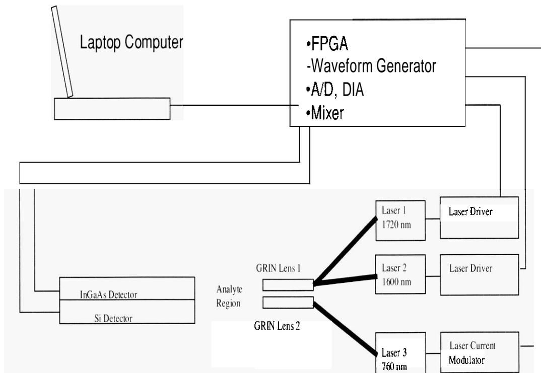
Figure 4. Component diagram of the binary gas sensor.
