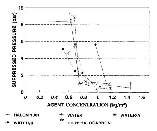
While water alone performs relatively poorly, water with inorganic additives performs very similarly to Halon 1301 and the best of the new halocarbons. Water is believed to be a highly attractive solution in these areas, providing the problem of freezing can be overcome or tolerated.
