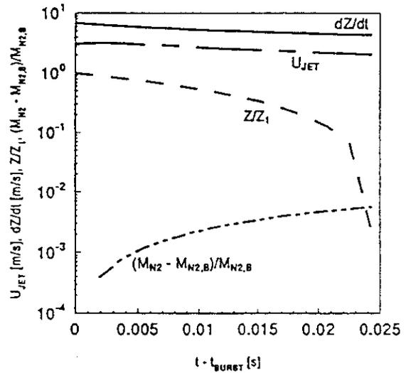
Figure 8. Plots of  $U_{JET}$ ,  $dZ/dt$ ,  $Z/Z_1$ , and  $(M_{N2} - M_{N2,B})/M_{N2,B}$  for  $t \geq t_{BURST}$ ; where  $V_{HT} = 2.5 \times 10^{-3} m^3$ ,  $T_{DV,1} = T_{HT,1} = 294K$ ,  $P_{DV,1} = P_{SAT} = 9.38 \times 10^5 Pa$  (136psi),  $P_{HT,1} = 51.71 \times 10^5 Pa$  (750psi),  $P_{BURST} = 37.92 \times 10^5 Pa$  (550psi) and  $D_O = 0.0005m$ .
