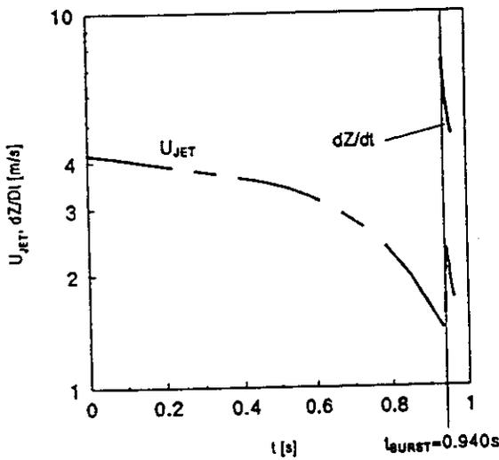
Figure 19. Plots of  $U_{JET}$  and  $dZ/dt$  for  $t \geq 0$  and  $D_O = 0.0005m$ ; where  $V_{HT} = 2.5 \times 10^{-5} m^3$ ,  $T_{DV,1} = T_{HT,1} = 294K$ ,  $P_{DV,1} = 34.47 \times 10^5 Pa$  (500psi),  $P_{HT,1} = 155.13 \times 10^5 Pa$  (2250psi),  $P_{BURST} = 44.82 \times 10^5 Pa$  (650psi).
