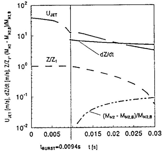
Figure 24. Plots of  $U_{JET}$ ,  $dZ/dt$ , and  $Z/Z_1$ , for  $t \geq 0$  and  $dZ/dt$ ,  $Z/Z_1$ , and of  $(M_{N2} - M_{N2,B})/M_{N2,B}$  for  $t \geq t_{BURST}$ ; where  $V_{HT} = 2.5 \times 10^{-5}\text{m}^3$ ,  $D_O = 0.005\text{m}$ ,  $T_{DV,1} = T_{HT,1} = 294\text{K}$ ,  $P_{DV,1} = 34.47 \times 10^5\text{Pa}$  (500psi),  $P_{HT,1} = 155.13 \times 10^5\text{Pa}$  (2250psi), and  $P_{BURST} = 44.82 \times 10^5\text{Pa}$  (650psi).
