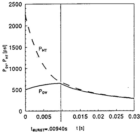
Figure 23. Plots of  $P_{DV}$  and  $P_{HT}$  for  $t \geq 0$  and  $D_O = 0.005\text{m}$ ; where  $V_{HT} = 2.5 \times 10^{-5}\text{m}^3$ ,  $T_{DV,1} = T_{HT,1} = 294\text{K}$ ,  $P_{DV,1} = 34.47 \times 10^5\text{Pa}$  (500psi),  $P_{HT,1} = 155.13 \times 10^5\text{Pa}$  (2250psi),  $P_{BURST} = 44.82 \times 10^5\text{Pa}$  (650psi).
