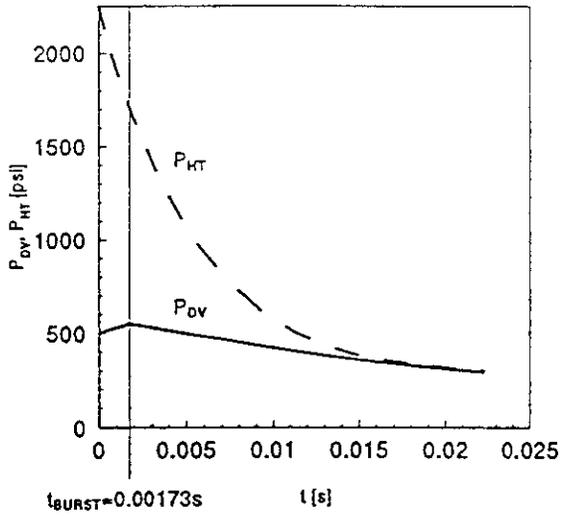
Figure 21. Plots of  $P_{DV}$  and  $P_{HT}$  for  $t \geq 0$  and  $D_O = 0.005\text{m}$ ; where  $V_{HT} = 2.5 \times 10^{-5}\text{m}^3$ ,  $T_{DV,1} = T_{HT,1} = 294\text{K}$ ,  $P_{DV,1} = 34.47 \times 10^5\text{Pa}$  (500psi),  $P_{HT,1} = 155.13 \times 10^5\text{Pa}$  (2250psi),  $P_{BURST} = 37.92 \times 10^5\text{Pa}$  (550psi).
