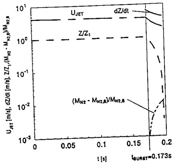
Figure 17. Plots of  $U_{JET}$ ,  $dZ/dt$ , and  $Z/Z_1$ , for  $t \geq 0$  and  $dZ/dt$ ,  $Z/Z_1$ , and of  $(M_{N2} - M_{N2,B})/M_{N2,B}$  for  $t \geq t_{BURST}$ ; where  $V_{HT} = 2.5 \times 10^{-5} m^3$ ,  $D_O = 0.0005m$ ,  $T_{DV,1} = T_{HT,1} = 294K$ ,  $P_{DV,1} = 34.47 \times 10^5 Pa$  (500psi),  $P_{HT,1} = 155.13 \times 10^5 Pa$  (2250psi), and  $P_{BURST} = 37.92 \times 10^5 Pa$  (550psi).
