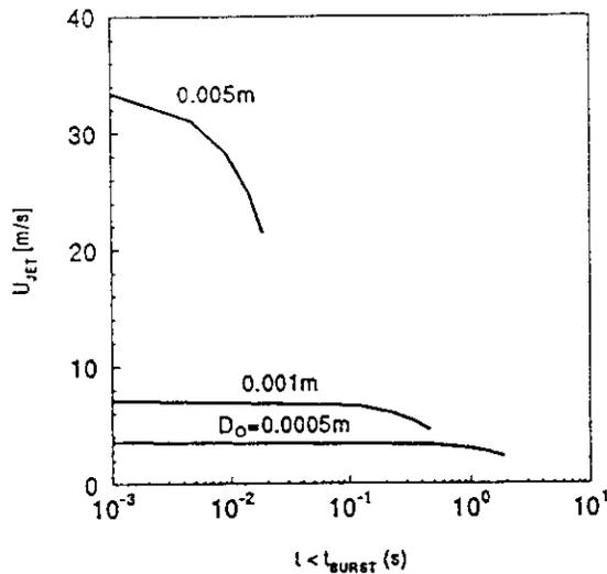
Figure 13. Plots of  $U_{JET}$  for  $0 \leq t \leq t_{BURST}$  and  $D_O = 0.005m, 0.001m,$  and  $0.0005m$ ; where  $V_{HT} = 2.5 \times 10^{-3} m^3$ ,  $T_{DV,1} = T_{HT,1} = 294K$ ,  $P_{DV,1} = 34.47 \times 10^5 Pa$  (500psi),  $P_{HT,1} = 51.71 \times 10^5 Pa$  (750psi),  $P_{BURST} \leq 44.82 \times 10^5 Pa$  (650psi).
