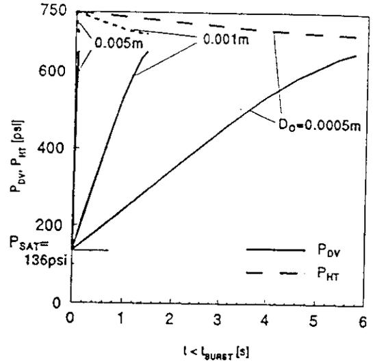
Figure 6. Plots of  $P_{DV}$  and  $P_{HT}$  for  $0 \leq t \leq t_{BURST}$  and  $D_O = 0.005m, 0.001m, \text{ and } 0.0005m$ ; where  $V_{HT} = 2.5 \times 10^{-3} m^3$ ,  $T_{DV,1} = T_{HT,1} = 294K$ ,  $P_{DV,1} = P_{SAT} = 9.38 \times 10^5 Pa$  (136psi),  $P_{HT,1} = 51.71 \times 10^5 Pa$  (750psi),  $P_{BURST} \leq 44.82 \times 10^5 Pa$  (650psi).
