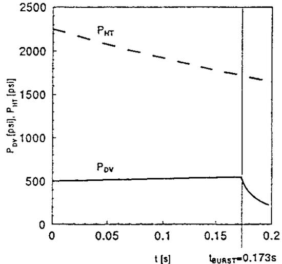
Figure 16. Plots of  $P_{DV}$  and  $P_{HT}$  for  $t \geq 0$  and  $D_O = 0.0005m$ ; where  $V_{HT} = 2.510^{-3} m^3$ ,  $T_{DV,1} = T_{HT,1} = 294K$ ,  $P_{DV,1} = 34.47 \times 10^5 Pa$  (500psi),  $P_{HT,1} = 155.13 \times 10^5 Pa$  (2250psi),  $P_{BURST} = 37.92 \times 10^5 Pa$  (550psi).
