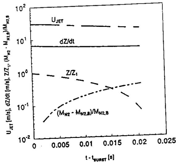
Figure 9. Plots of  $U_{JET}$ ,  $dZ/dt$ ,  $Z/Z_1$ , and  $(M_{N2} - M_{N2,B})/M_{N2,B}$  for  $t \geq t_{BURST}$ ; where  $V_{HT} = 2.5 \times 10^{-3} \text{m}^3$ ,  $T_{DV,1} = T_{HT,1} = 294 \text{K}$ ,  $P_{DV,1} = P_{SAT} = 9.38 \times 10^5 \text{Pa}$  (136psi),  $P_{HT,1} = 51.71 \times 10^5 \text{Pa}$  (750psi),  $P_{BURST} = 37.92 \times 10^5 \text{Pa}$  (550psi) and  $D_0 = 0.005 \text{m}$ .
