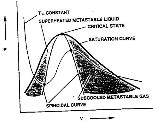
Figure 2. P-V diagram for a generic material; the spinoidal curve and regions of metastable liquid and vapor.
