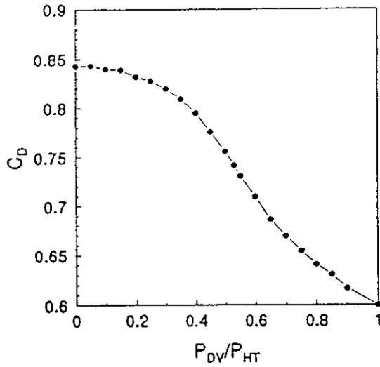
Figure 5. Discharge coefficient,  $C_{D,O}$ , for compressible flow through a sharp-edged orifice as a function of cross-orifice pressure ratio,  $P_{DV}/P_{HT}$  [11].
