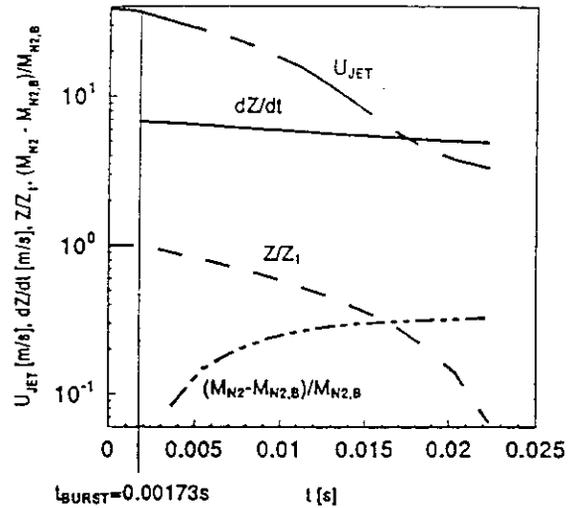
Figure 22. Plots of  $U_{JET}$ ,  $dZ/dt$ , and  $Z/Z_1$ , for  $t \geq 0$  and  $dZ/dt$ ,  $Z/Z_1$ , and of  $(M_{N2} - M_{N2,B})/M_{N2,B}$  for  $t \geq t_{BURST}$ ; where  $V_{HT} = 2.5 \times 10^{-5}\text{m}^3$ ,  $D_O = 0.005\text{m}$ ,  $T_{DV,1} = T_{HT,1} = 294\text{K}$ ,  $P_{DV,1} = 34.47 \times 10^5\text{Pa}$  (500psi),  $P_{HT,1} = 155.13 \times 10^5\text{Pa}$  (2250psi), and  $P_{BURST} = 37.92 \times 10^5\text{Pa}$  (550psi).
