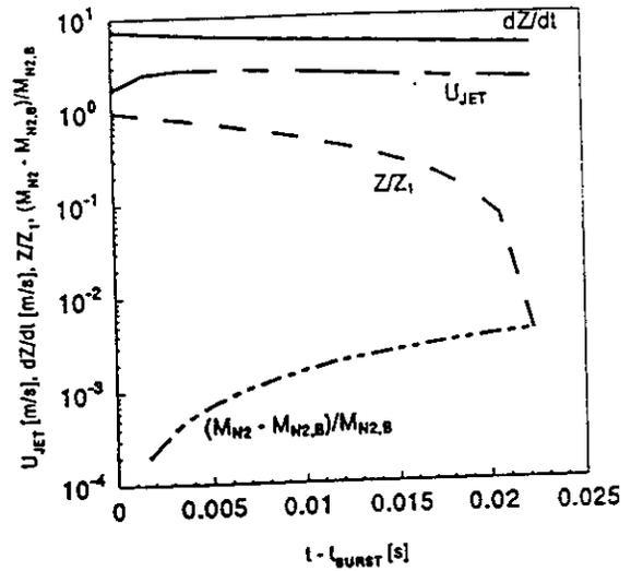
Figure 10. Plots of  $U_{JET}$ ,  $dZ/dt$ ,  $Z/Z_1$ , and  $(M_{N2} - M_{N2,B})/M_{N2,B}$  for  $t \geq t_{BURST}$ ; where  $V_{HT} = 2.5 \times 10^{-3} \text{m}^3$ ,  $T_{DV,1} = T_{HT,1} = 294 \text{K}$ ,  $P_{DV,1} = P_{SAT} = 9.38 \times 10^5 \text{Pa}$  (136psi),  $P_{HT,1} = 51.71 \times 10^5 \text{Pa}$  (750psi),  $P_{BURST} = 44.82 \times 10^5 \text{Pa}$  (650psi) and  $D_0 = 0.0005 \text{m}$ .
