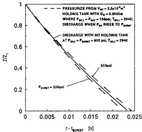
Figure 15. Plots of  $Z/Z_1$  during discharge of: 1) field-deployed vessel at  $P_{BURST} = 41.37 \times 10^5 Pa$  (600psi) and test configuration vessel [ $V_{HT} = 2.510^{-3} m^3$ ,  $D_O = 0.0005m$ ,  $P_{DV,1} = P_{SAT}(294K) = 9.38 \times 10^5 Pa$  (136psi)] at 2)  $P_{BURST} = 37.92 \times 10^5 Pa$  (550psi) and 3)  $44.82 \times 10^5 Pa$  (650psi).
