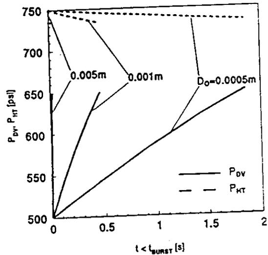
Figure 12. Plots of  $P_{DV}$  and  $P_{HT}$  for  $0 \leq t \leq t_{BURST}$  and  $D_0 = 0.005 \text{m}$ ,  $0.001 \text{m}$ , and  $0.0005 \text{m}$ ; where  $V_{HT} = 2.5 \times 10^{-3} \text{m}^3$ ,  $T_{DV,1} = T_{HT,1} = 294 \text{K}$ ,  $P_{DV,1} = 34.47 \times 10^5 \text{Pa}$  (500psi),  $P_{HT,1} = 51.71 \times 10^5 \text{Pa}$  (750psi),  $P_{BURST} \leq 44.82 \times 10^5 \text{Pa}$  (650psi).
