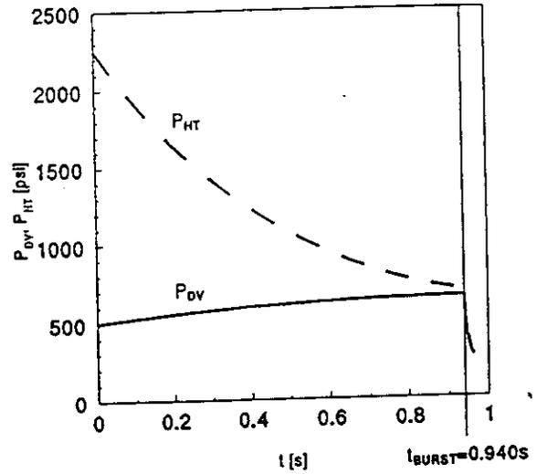
Figure 18. Plots of  $P_{DV}$  and  $P_{HT}$  for  $t \geq 0$  and  $D_O = 0.0005m$ ; where  $V_{HT} = 2.5 \times 10^{-5} m^3$ ,  $T_{DV,1} = T_{HT,1} = 294K$ ,  $P_{DV,1} = 34.47 \times 10^5 Pa$  (500psi),  $P_{HT,1} = 155.13 \times 10^5 Pa$  (2250psi),  $P_{BURST} = 44.82 \times 10^5 Pa$  (650psi).
