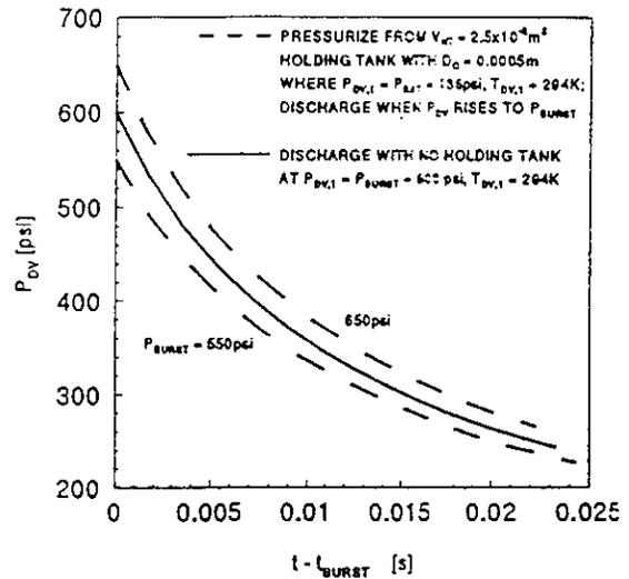
Figure 14. Plots of  $P_{DV}$  during discharge of: 1) field-deployed vessel at  $P_{BURST} = 41.37 \times 10^5 Pa$  (600psi) and test configuration vessel [ $V_{HT} = 2.5 \times 10^{-3} m^3$ ,  $D_O = 0.0005m$ ,  $P_{DV,1} = P_{SAT}(294K) = 9.38 \times 10^5 Pa$  (136psi)] at 2)  $P_{BURST} = 37.92 \times 10^5 Pa$  (550psi) and 3)  $44.82 \times 10^5 Pa$  (650psi).
