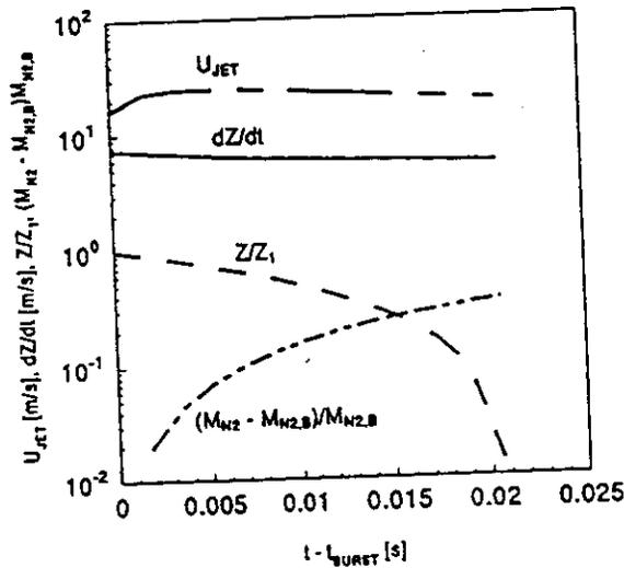
Figure 11. Plots of  $U_{JET}$ ,  $dZ/dt$ ,  $Z/Z_1$ , and  $(M_{N2} - M_{N2,B})/M_{N2,B}$  for  $t \geq t_{BURST}$ ; where  $V_{HT} = 2.5 \times 10^{-3} \text{m}^3$ ,  $T_{DV,1} = T_{HT,1} = 294 \text{K}$ ,  $P_{DV,1} = P_{SAT} = 9.38 \times 10^5 \text{Pa}$  (136psi),  $P_{HT,1} = 51.71 \times 10^5 \text{Pa}$  (750psi),  $P_{BURST} = 44.82 \times 10^5 \text{Pa}$  (650psi) and  $D_0 = 0.005 \text{m}$ .
