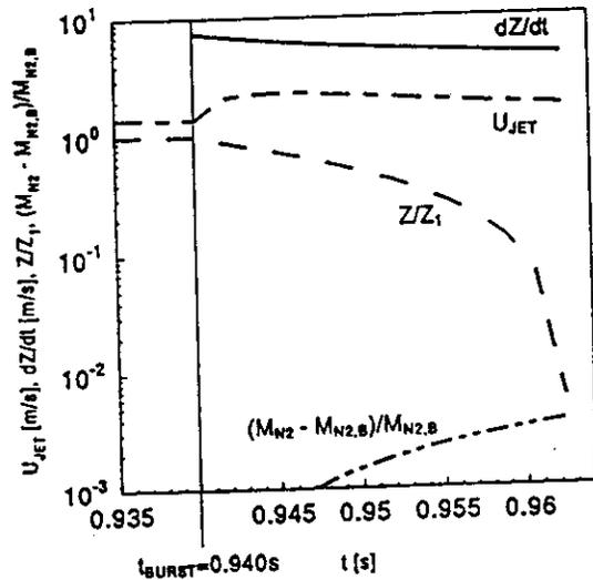
Figure 20. Plots of  $U_{JET}$ ,  $dZ/dt$ ,  $Z/Z_1$ , and  $(M_{N2} - M_{N2,B})/M_{N2,B}$  for  $t \geq t_{BURST}$  and  $D_O = 0.0005m$ ; where  $V_{HT} = 2.5 \times 10^{-5} m^3$ ,  $T_{DV,1} = T_{HT,1} = 294K$ ,  $P_{DV,1} = 34.47 \times 10^5 Pa$  (500psi),  $P_{HT,1} = 155.13 \times 10^5 Pa$  (2250psi), and  $P_{BURST} = 44.82 \times 10^5 Pa$  (650psi).
