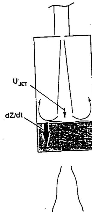
Figure 4. Sketch of the orifice-driven N<sub>2</sub> jet flow in the discharge vessel.
