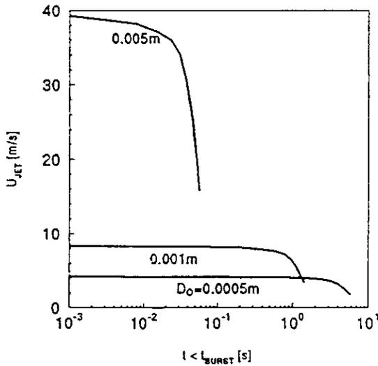
Figure 7. Plots of  $U_{JET}$  for  $0 \leq t \leq t_{BURST}$  and  $D_O = 0.005m, 0.001m, \text{ and } 0.0005m$ ; where  $V_{HT} = 2.5 \times 10^{-3} m^3$ ,  $T_{DV,1} = T_{HT,1} = 294K$ ,  $P_{DV,1} = P_{SAT} = 9.38 \times 10^5 Pa$  (136psi),  $P_{HT,1} = 51.71 \times 10^5 Pa$  (750psi),  $P_{BURST} \leq 44.82 \times 10^5 Pa$  (650psi).
