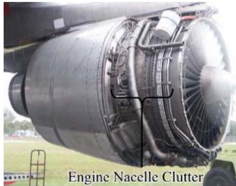
**Figure 1. Typical aircraft engine nacelle clutter.**
