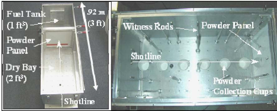
Figure 1. Experimental Test Device and Powder Collection Methods
