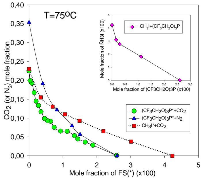
**Figure 1. Cup burner tests: extinguishing concentration of CO<sub>2</sub> as a function of loading of fire suppressants.**
