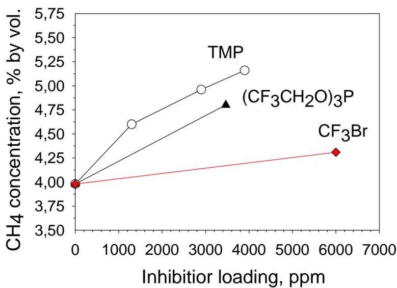
**Figure 6. The dependence of lean flammability limits of CH<sub>4</sub>/Air mixtures on inhibitors loading.**
