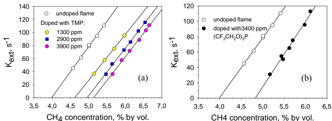
**Figure 5. Global extinction strain rates  $K_{ext}$  versus CH<sub>4</sub> concentration [CH<sub>4</sub>] for lean premixed CH<sub>4</sub>/Air counterflow flames doped with TMP (a) and (CF<sub>3</sub>CH<sub>2</sub>O)<sub>3</sub>P (b), and without additives.**
