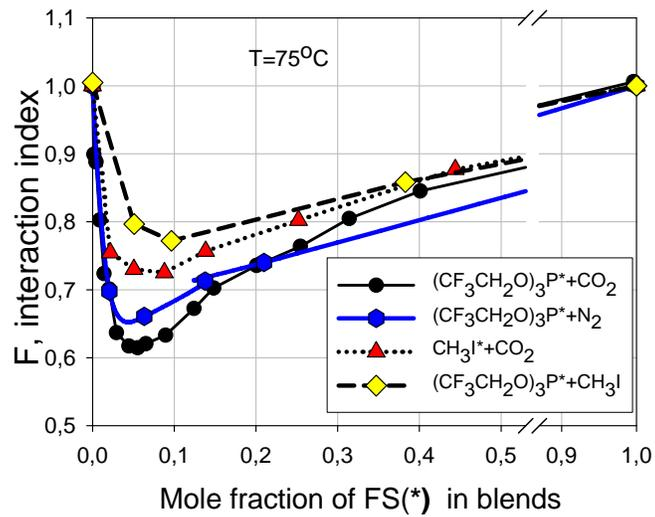
**Figure 2. Interaction index for blends (CF<sub>3</sub>CH<sub>2</sub>O)<sub>3</sub>P with CO<sub>2</sub>, N<sub>2</sub> or CH<sub>3</sub>I.**
