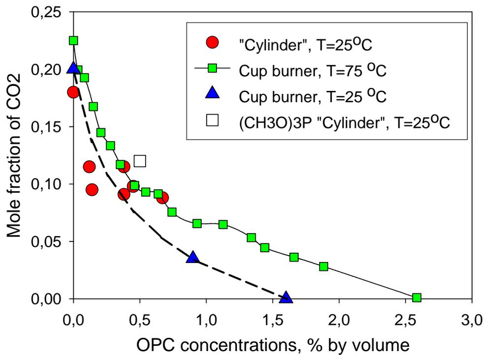
**Figure 4. Comparison of extinguishing concentrations obtained by using cup-burner and “cylinder” technique for blends of CO<sub>2</sub> with (CF<sub>3</sub>CH<sub>2</sub>O)<sub>3</sub>P.**
