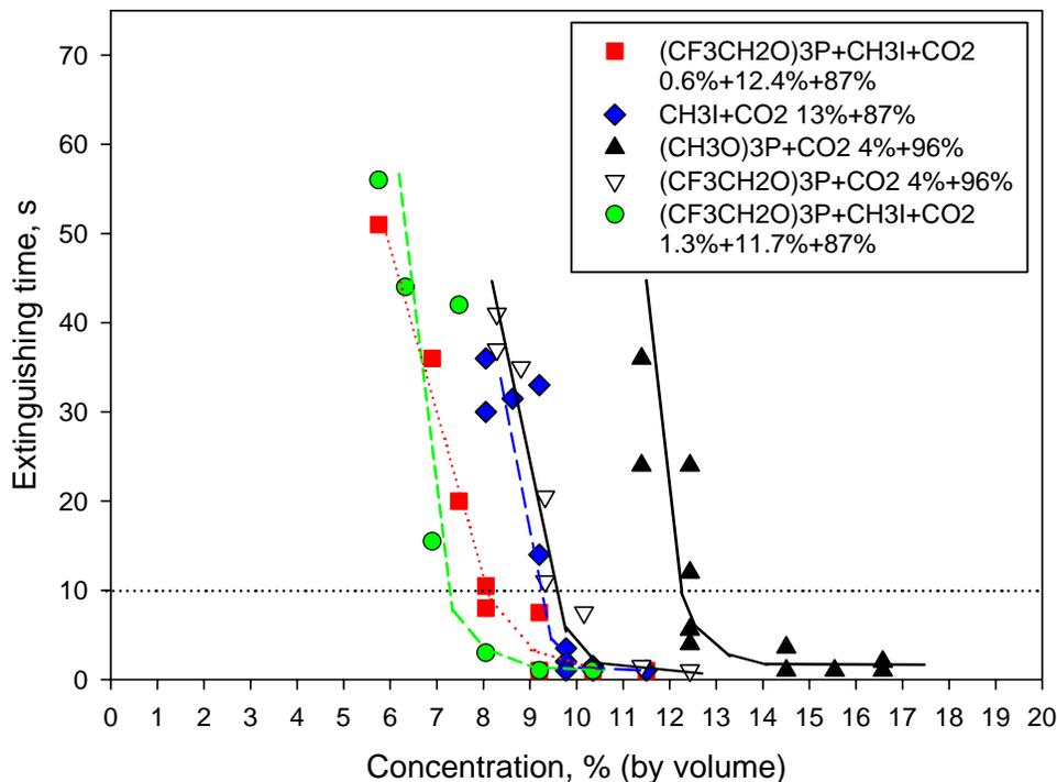
**Figure 3. Typical dependencies of time of extinguishing on a volume concentration of blends.**
